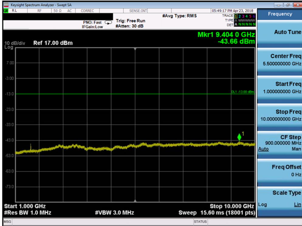
Plot 7-13. Conducted Spurious Plot (LTE B14 – 5.0MHz QPSK – RB Size 1, RB Offset 0 – High Channel)
