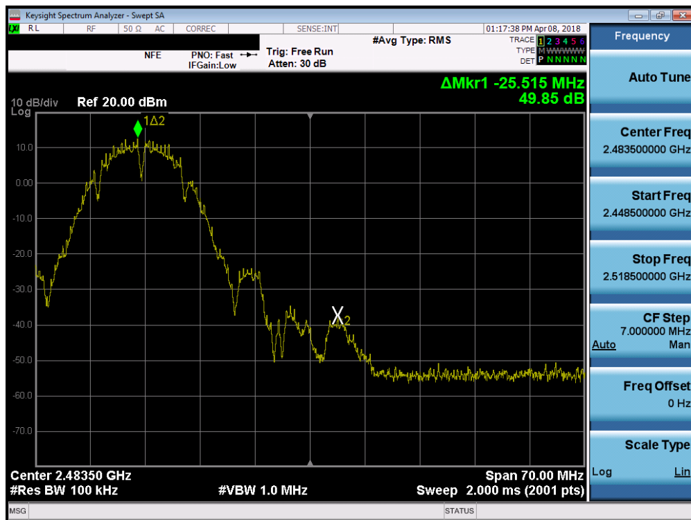
Plot 7-20. Band Edge Plot (802.11b – Ch. 11)
