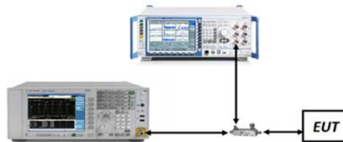
Figure 7-3. Test Instrument & Measurement Setup
