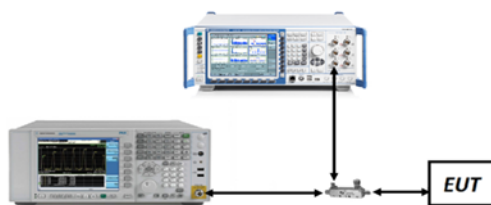
Figure 7-1. Test Instrument & Measurement Setup
