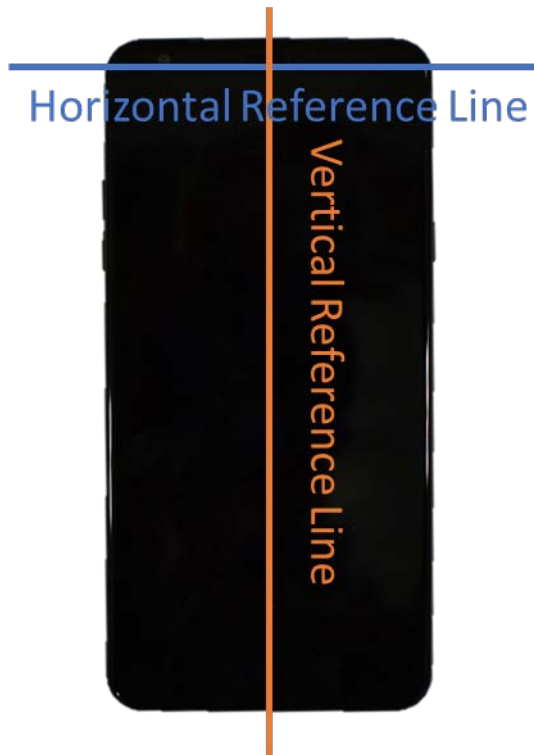
SAR Test Setup Photo 17 – Vertical and Horizontal Reference lines
