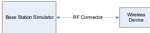
Figure 9-2 Power Measurement Setup
