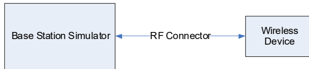
Figure 9-1 Power Measurement Setup
