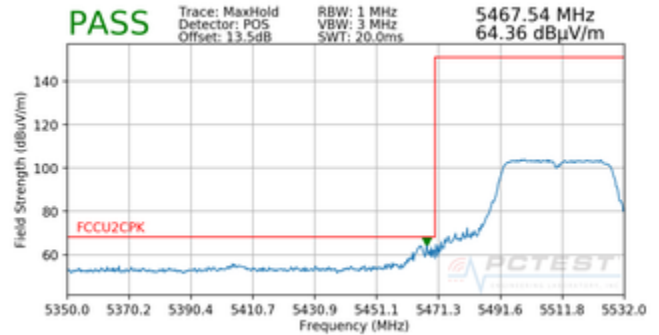
Plot 7-91. Radiated Lower Band Edge Plot (Peak – UNII Band 2C)
