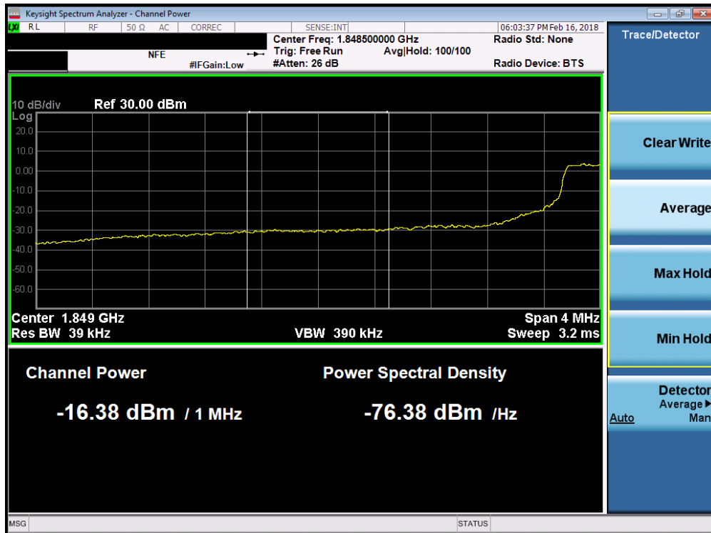
Plot 7-225. Lower Extended Band Edge Plot (Band 2 - 5.0MHz QPSK - Full RB Configuration)
