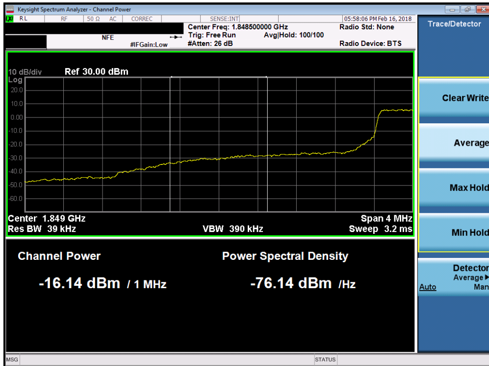
Plot 7-221. Lower Extended Band Edge Plot (Band 2 - 3.0MHz QPSK - Full RB Configuration)
