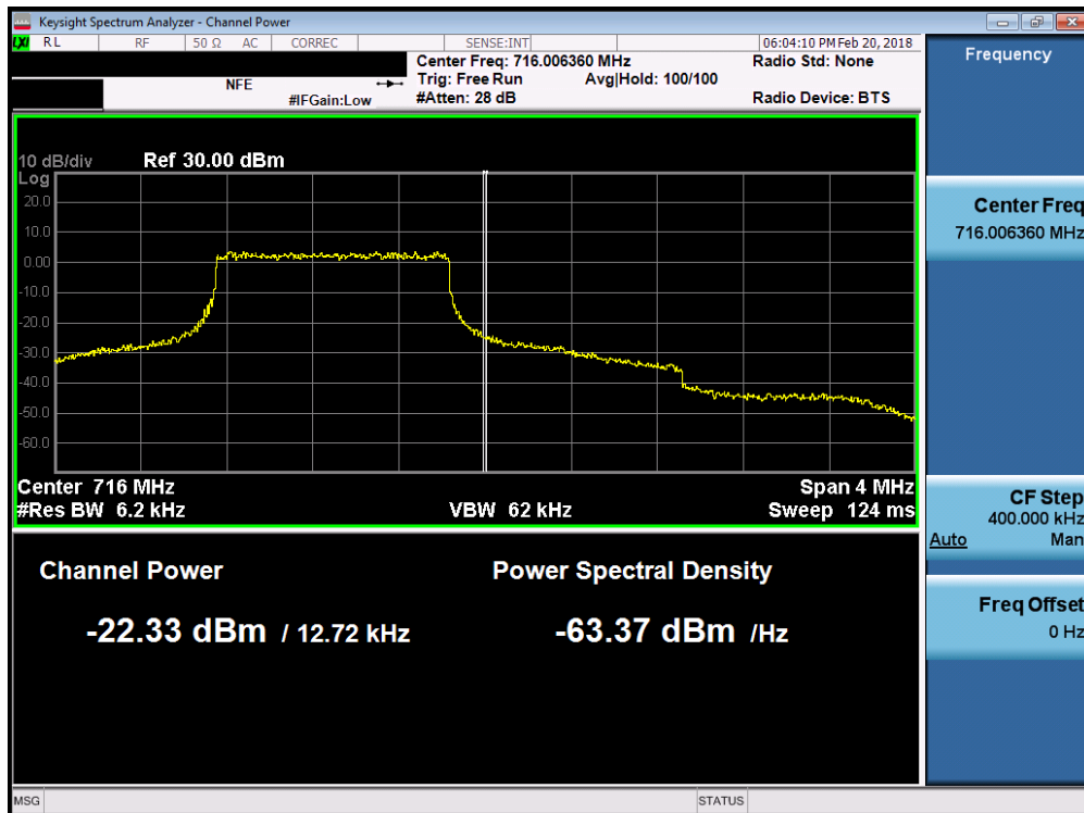
Plot 7-157. Upper Band Edge Plot (Band 12 - 1.4MHz QPSK - Full RB Configuration)
