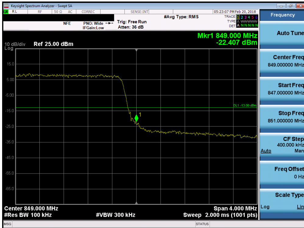
Plot 7-177. Upper Band Edge Plot (Band 5 - 5.0MHz QPSK - Full RB Configuration)
