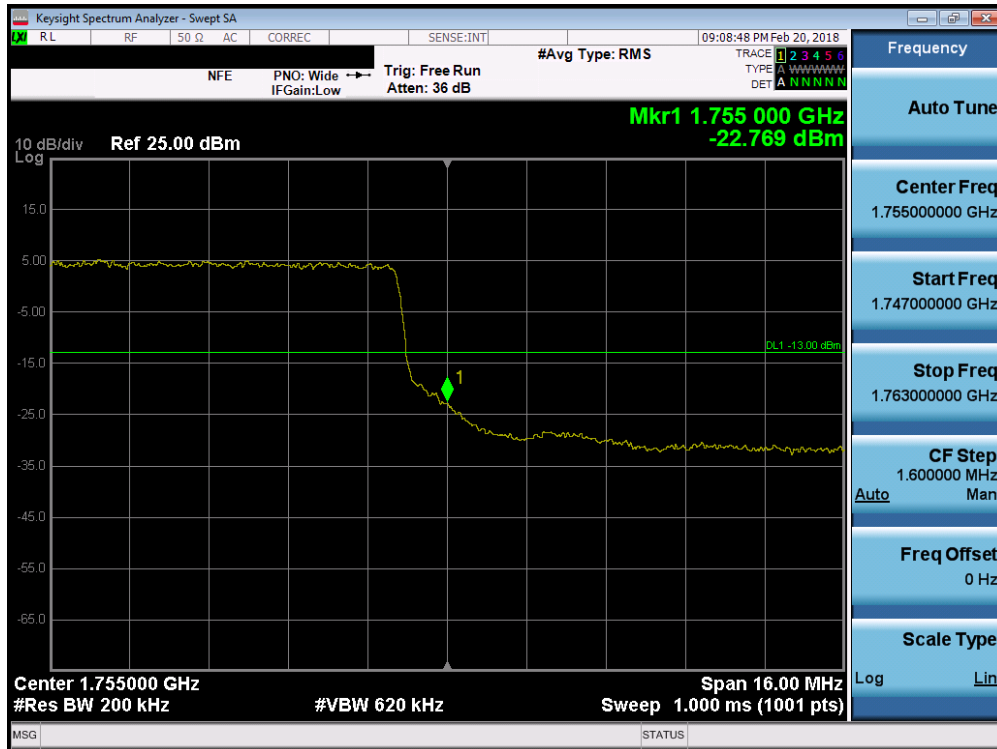
Plot 7-212. Upper Band Edge Plot (Band 4 - 20.0MHz QPSK - Full RB Configuration)
