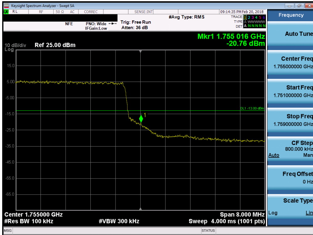
Plot 7-200. Upper Band Edge Plot (Band 4 - 10.0MHz QPSK - Full RB Configuration)
