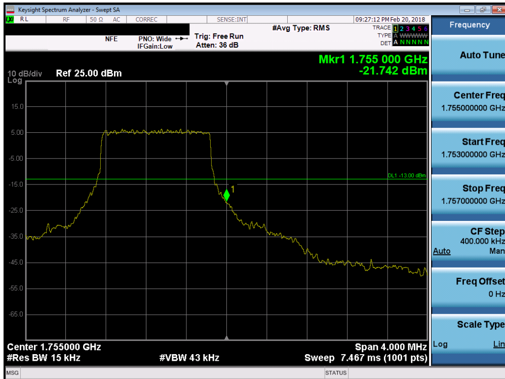
Plot 7-182. Upper Band Edge Plot (Band 4 - 1.4MHz QPSK - Full RB Configuration)
