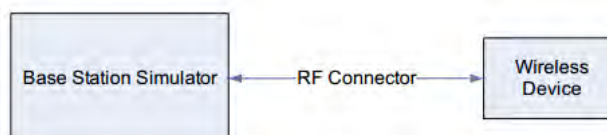
Figure 10.1 Power Measurement Setup
