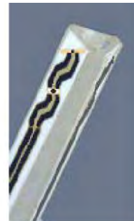
Figure 3.3 Probe Thick-Film Technique
