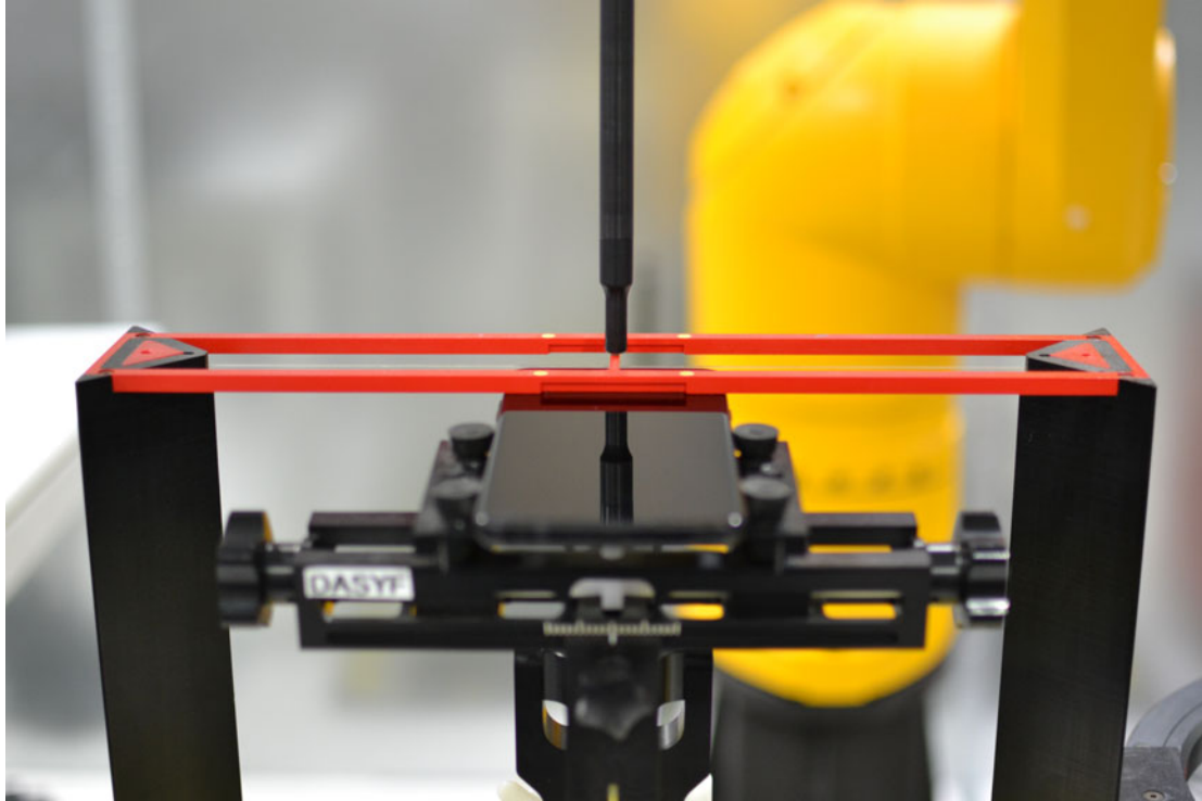
Figure 17-1 Ear Reference Point HAC Phantom Alignment
