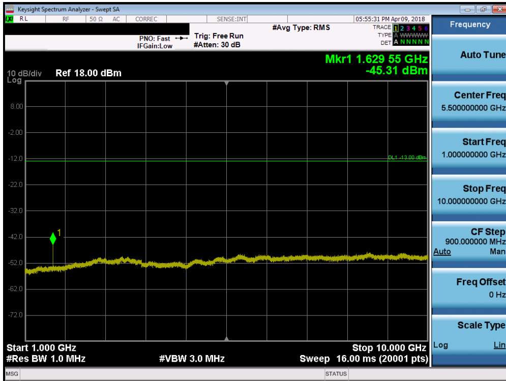
Plot 7-21. Conducted Spurious Plot (LTE B26 - 1.4MHz QPSK – RB Size 1, RB Offset 0 – Low Channel)
