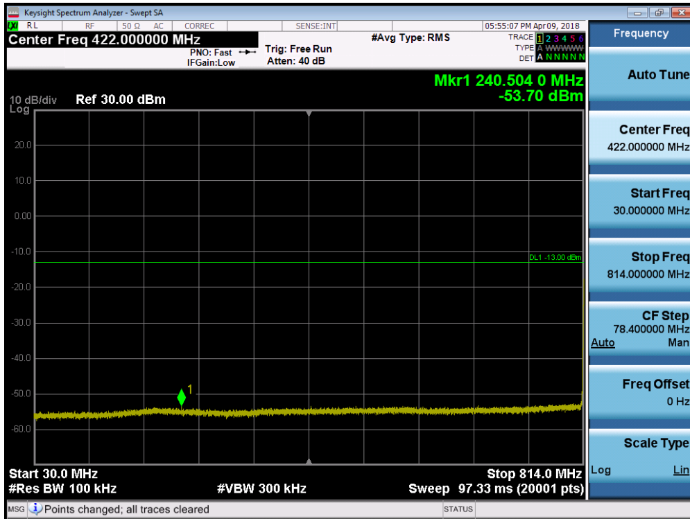
Plot 7-19. Conducted Spurious Plot (LTE B26 - 1.4MHz QPSK – RB Size 1, RB Offset 0 – Low Channel)
