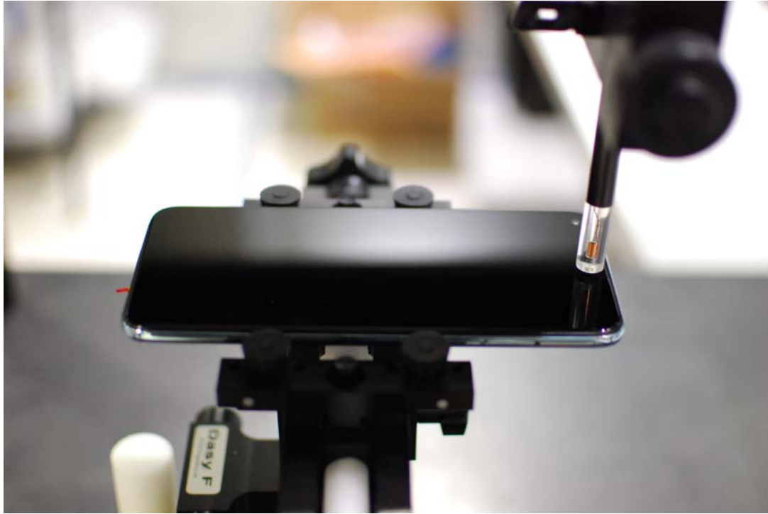
Figure 16-1 Test Setup for Wireless Device
