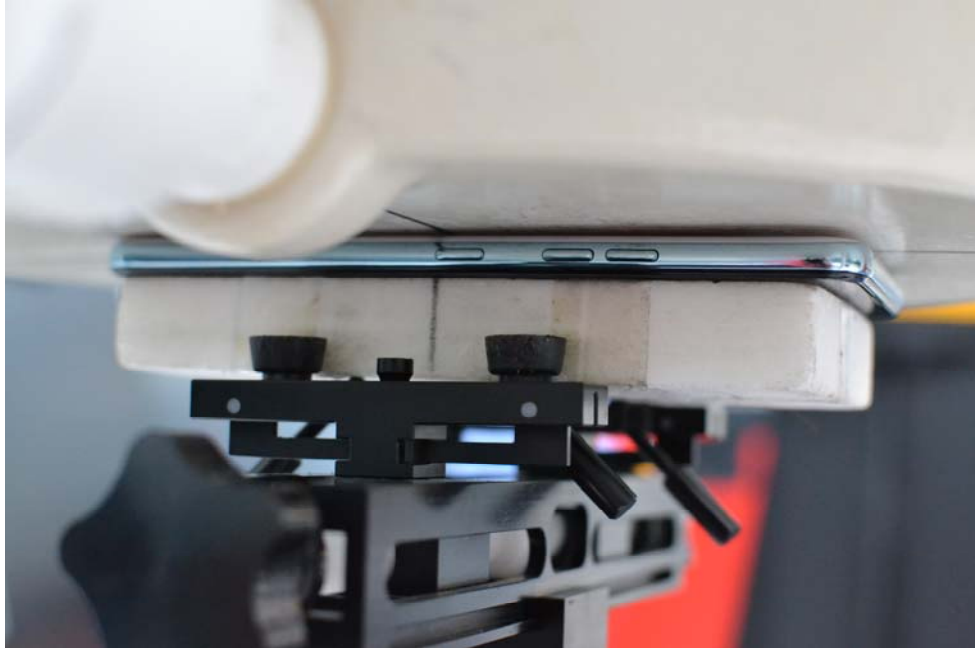
SAR Test Setup Photo 12: Back at 0 mm
