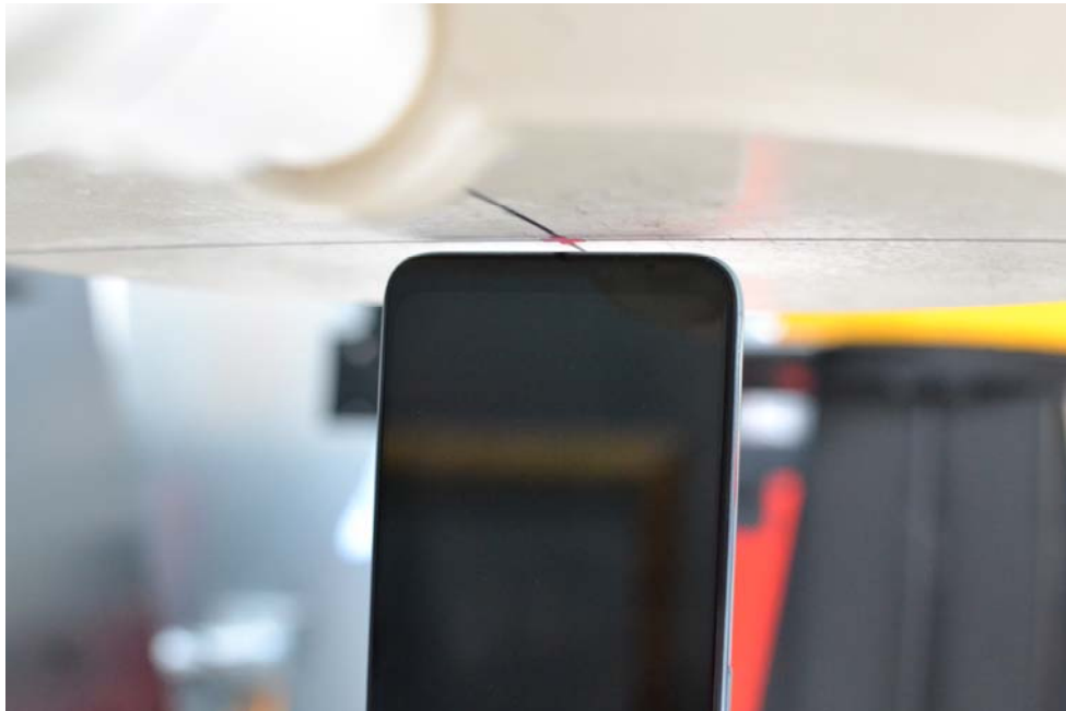
SAR Test Setup Photo 15: Bottom at 3 mm
