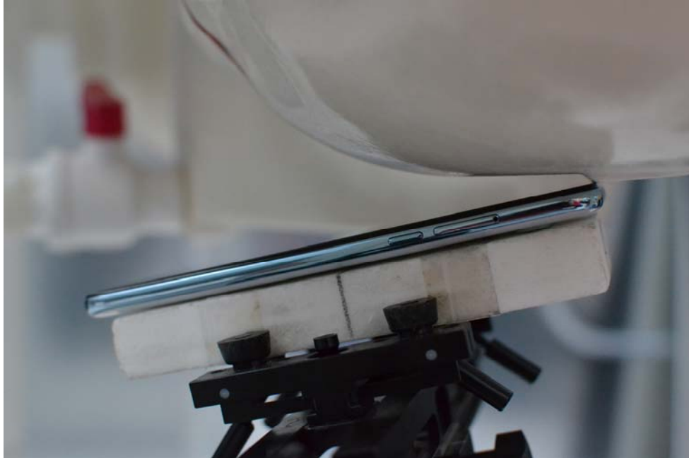
SAR Test Setup Photo 4: Left Tilt
