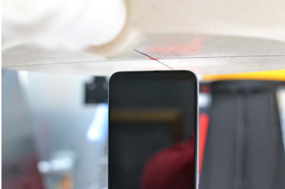
SAR Test Setup Photo 8: Bottom at 10 mm
