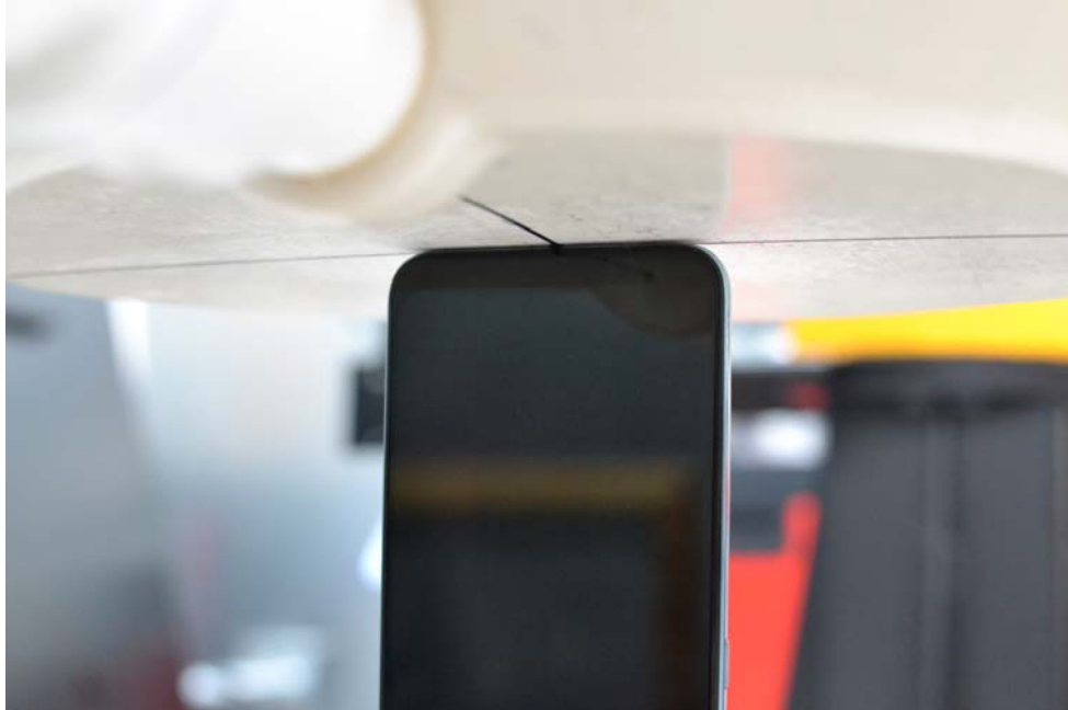
SAR Test Setup Photo 16: Bottom at 0 mm
