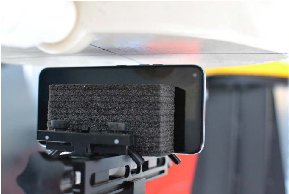
SAR Test Setup Photo 10: Left at 10 mm
