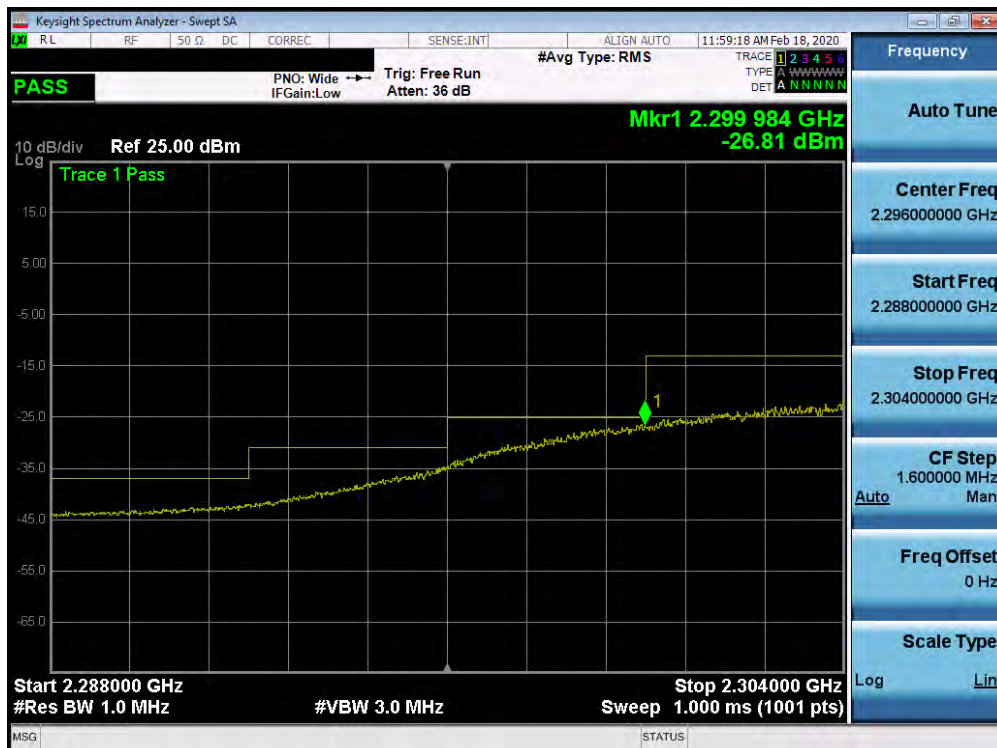
Plot 7-211. Lower Extended Band Edge Plot (Band 30 - 10.0MHz QPSK - Full RB Configuration)
