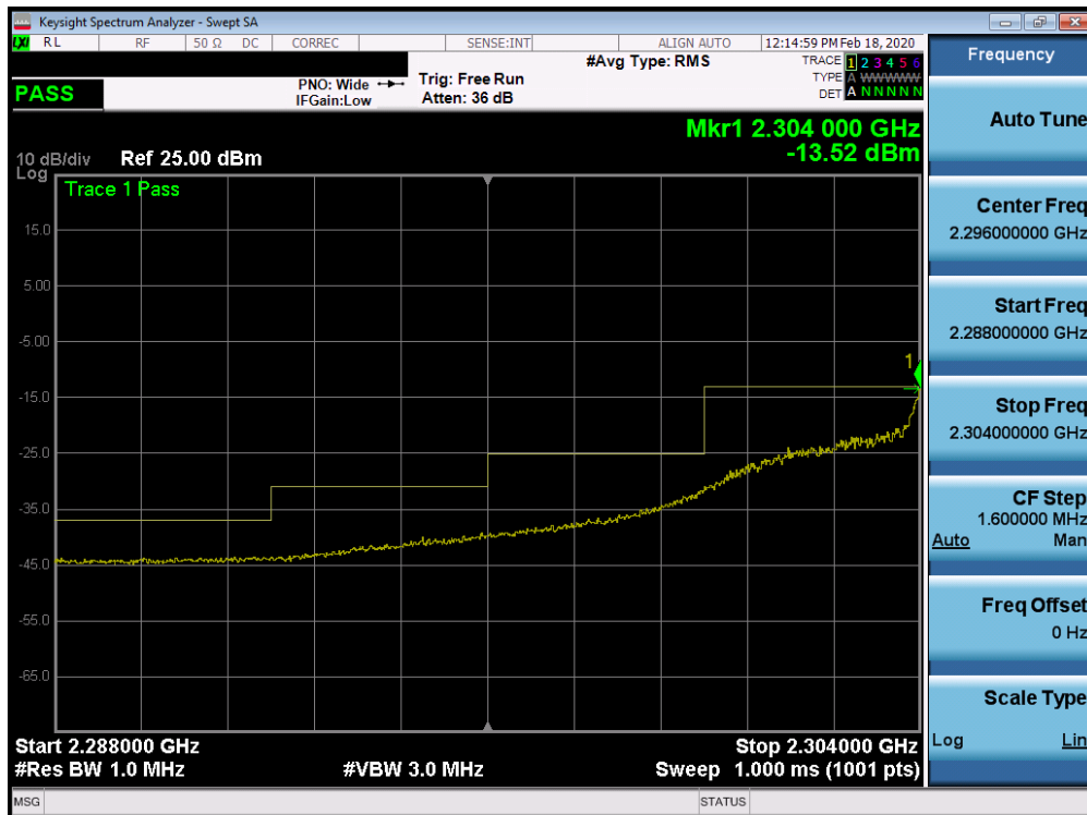
Plot 7-207. Lower Extended Band Edge Plot (Band 30 - 5.0MHz QPSK - Full RB Configuration)
