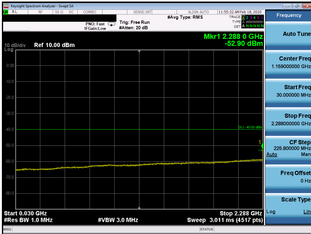
Plot 7-96. Conducted Spurious Plot (Band 30 - 10.0MHz QPSK - RB Size 1, RB Offset 0 - Mid Channel)
