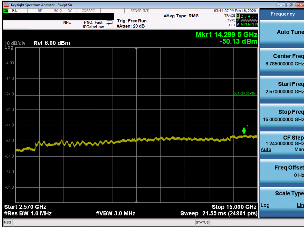
Plot 7-103. Conducted Spurious Plot (Band 7 - 20.0MHz QPSK - RB Size 1, RB Offset 0 - Mid Channel)
