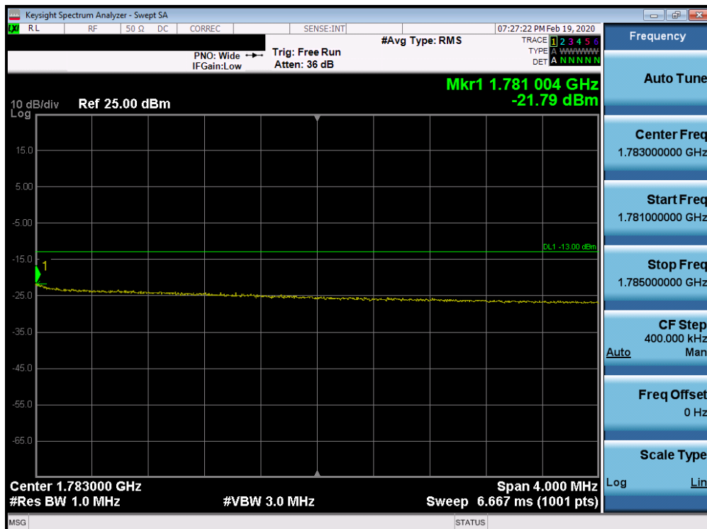
Plot 7-157. Upper Extended Band Edge Plot (Band 66 - 10.0MHz QPSK - Full RB Configuration)
