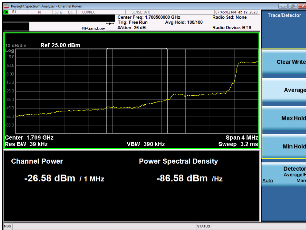
Plot 7-135. Lower Extended Band Edge Plot (Band 66/4 - 1.4MHz QPSK - Full RB Configuration)
