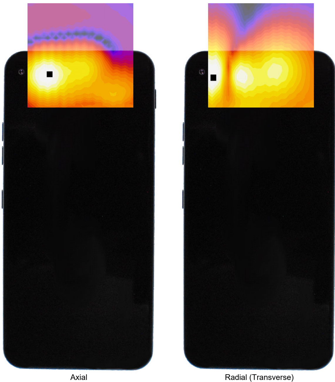
Figure 16-3 T-Coil Scan Overlay Magnetic Field Distributions
