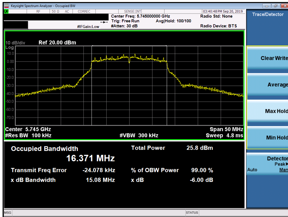
Plot 7-31. 6dB Bandwidth Plot (802.11a (UNII Band 3) – Ch. 149)
