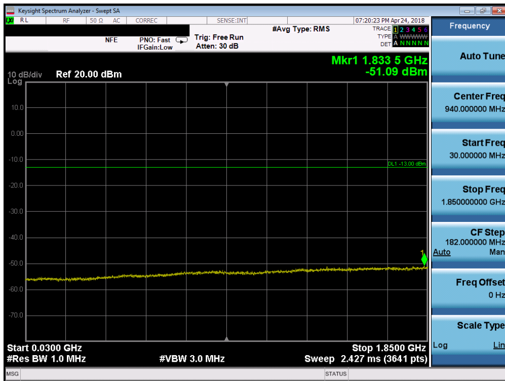
Plot 7-133. Conducted Spurious Plot (Band 2 - 10.0MHz QPSK - RB Size 1, RB Offset 0 - Mid Channel)
