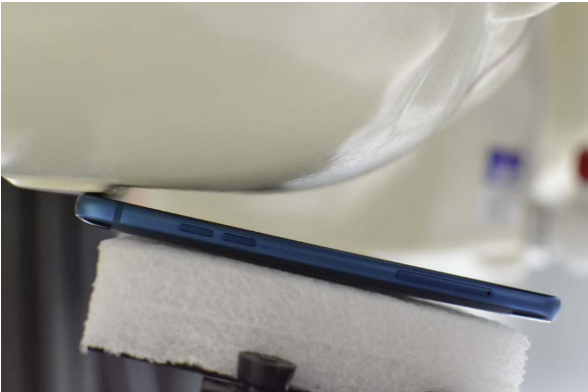
SAR Test Setup Photo 2: Right Tilt
