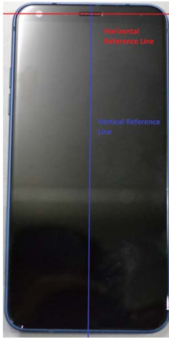
SAR Test Setup Photo 11: Vertical and Horizontal Reference Lines
