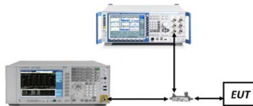
Figure 7-2. Test Instrument & Measurement Setup
