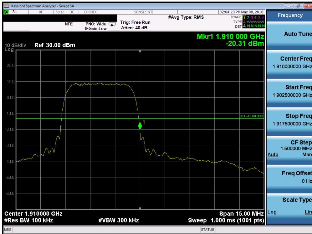
Plot 7-67. Band Edge Plot (PCS WCDMA Mode - High Channel)
