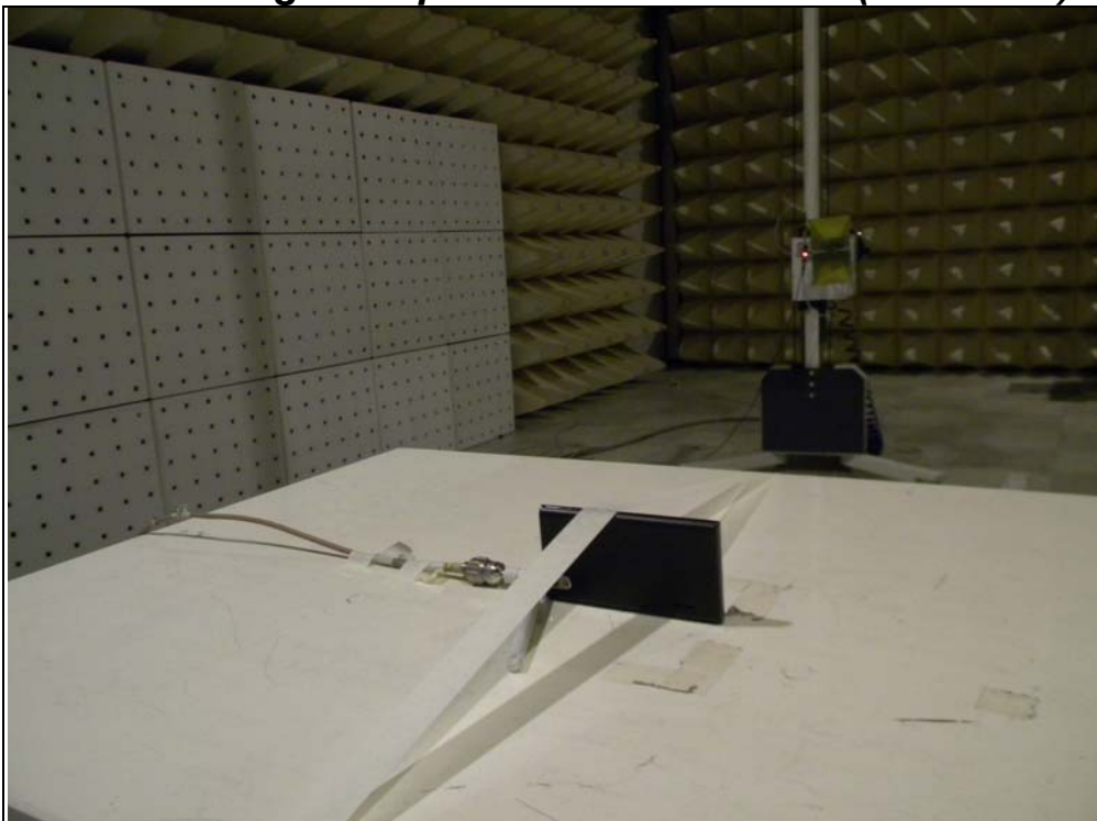
B. Photo of Field Strength & Spurious Emission Test(2G/3G/BT)
