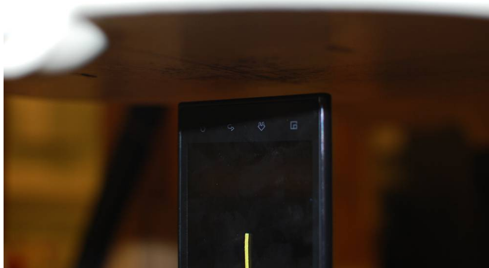
SAR Test Setup Photo 8 – Bottom at 1.0 cm
