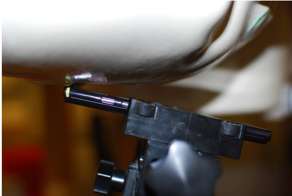
SAR Test Setup Photo 2 – Right Tilt
