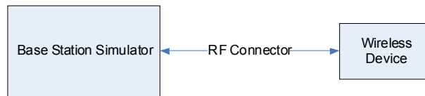
Figure 11-1 Power Measurement Setup
