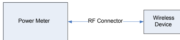
Figure 12-1 Power Measurement Setup
