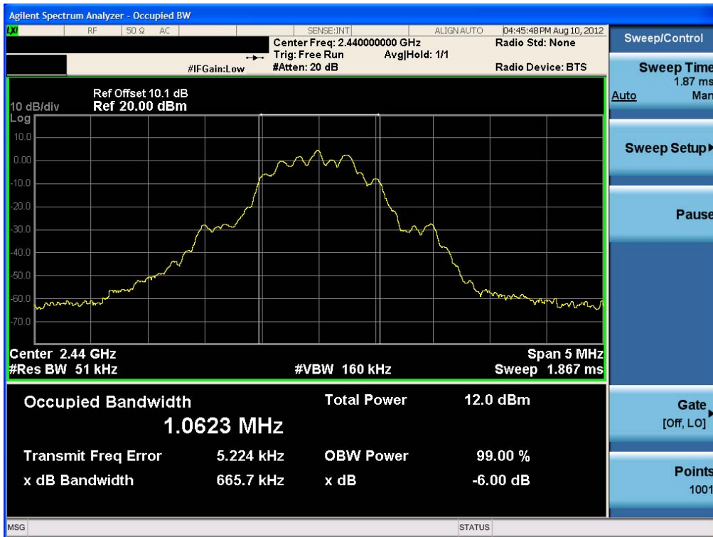
6dB Bandwidth plot (Mid-CH 19)
