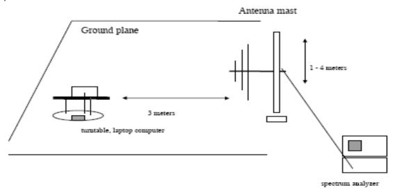
Test Procedures: Radiated emissions were measured according to ANSI C63.4.
