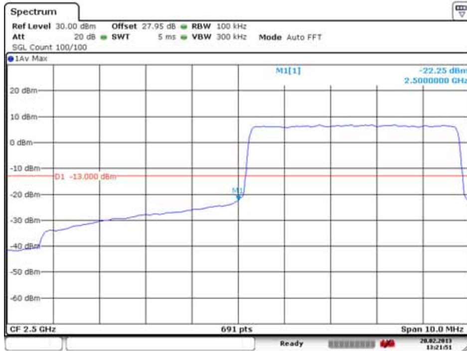
Low Band Edge Plot (20775 ch_5 MHz_QPSK_RB 25_0)
