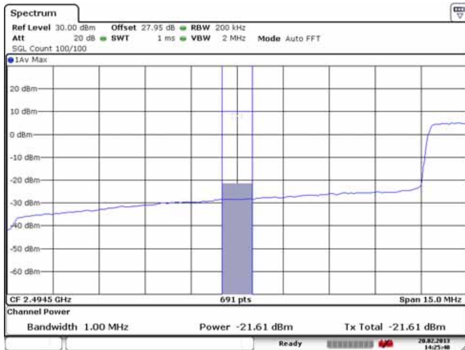
Low Extended Band Edge Plot (20825_15 MHz_QPSK_RB 75_0)
