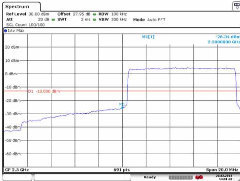
Low Band Edge Plot (20800 ch_10 MHz_QPSK_RB 50_0)
