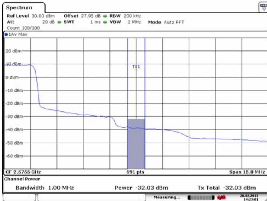
High Extended Band Edge Plot (21425 ch_5 MHz_QPSK_RB 25_0)
