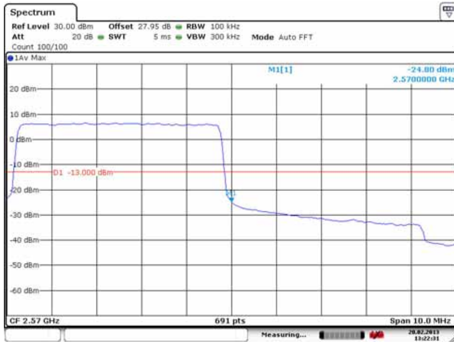
High Band Edge Plot (21425 ch_5 MHz_QPSK_RB 25_0)
