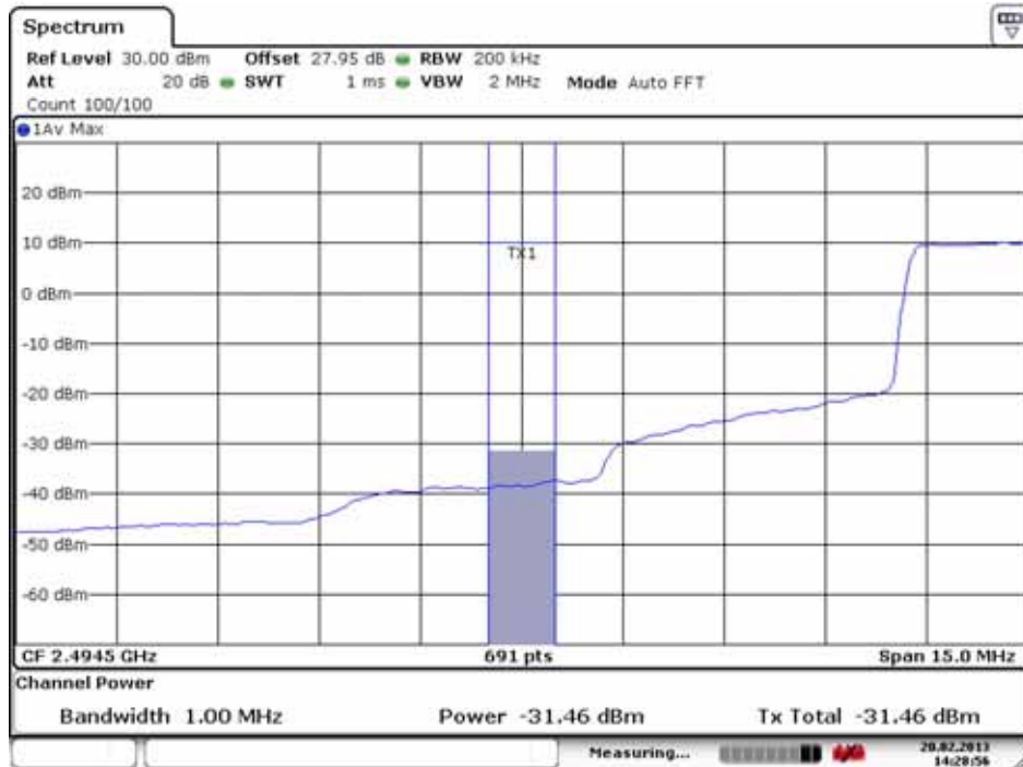
Low Extended Band Edge Plot (20775_5 MHz_QPSK_RB 25_0)
