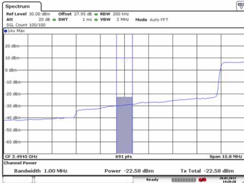
Low Extended Band Edge (20800 ch_10 MHz_QPSK_RB 50_0)
