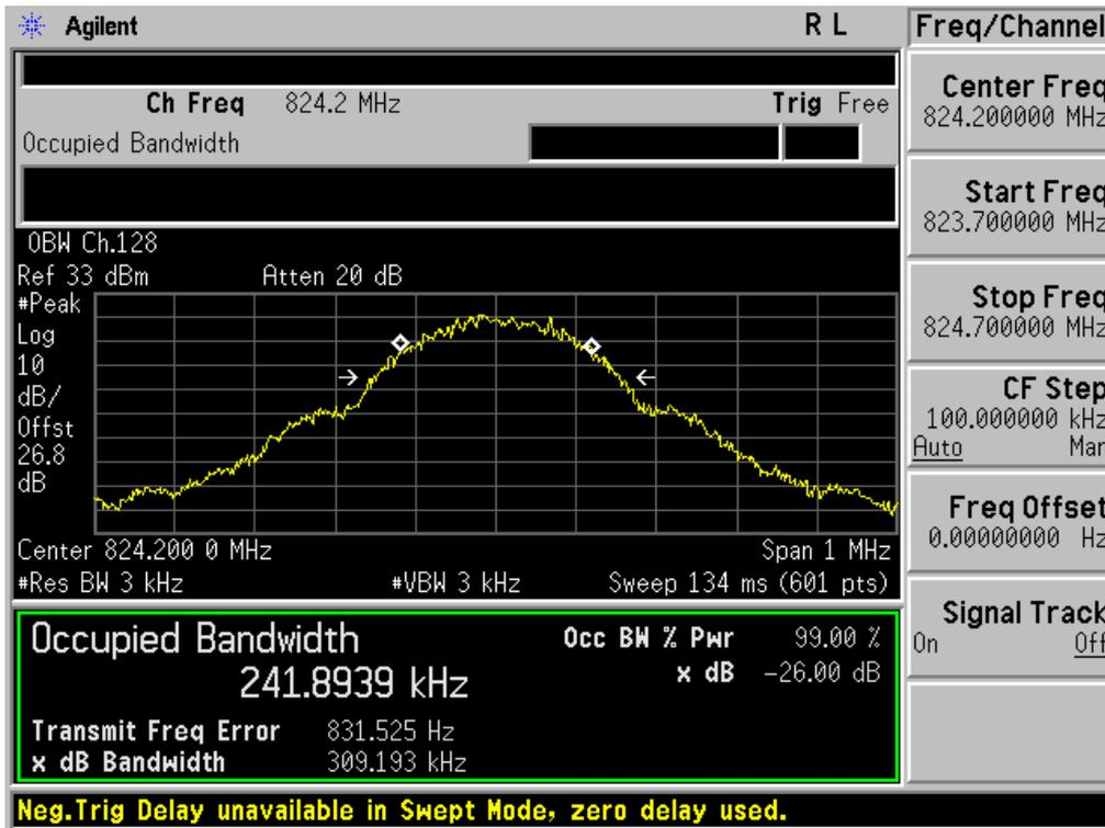
■ GSM850 MODE (190 CH.) Occupied Bandwidth
