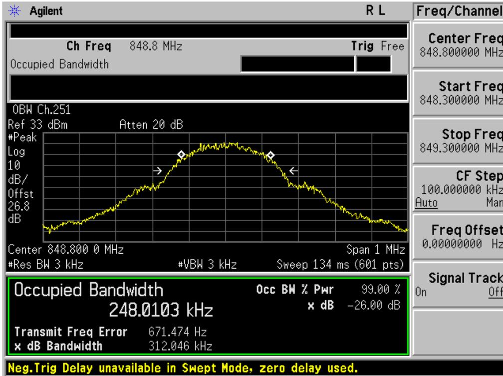
■ GSM850 EDGE (251 CH.) Occupied Bandwidth
