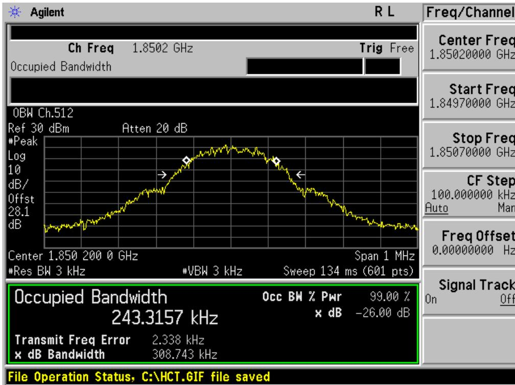
■ GSM1900 MODE (661 CH.) Occupied Bandwidth
