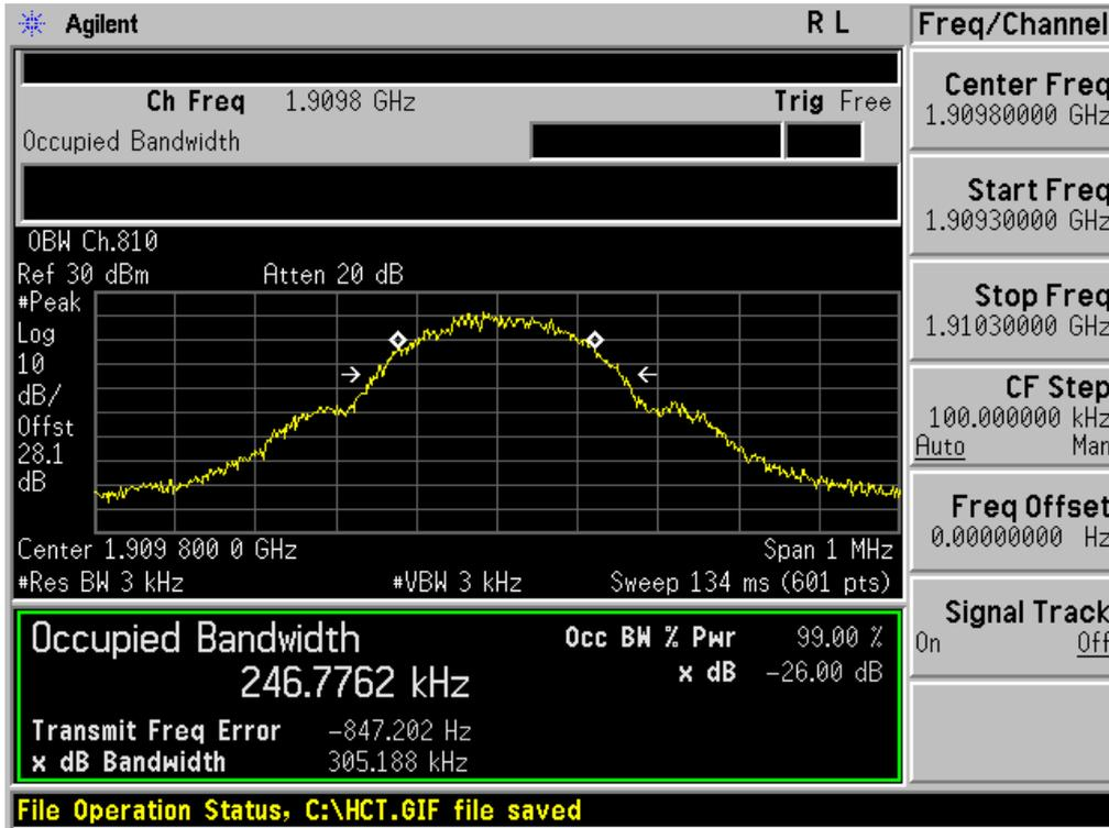
■ GSM1900 EDGE (810 CH.) Occupied Bandwidth
