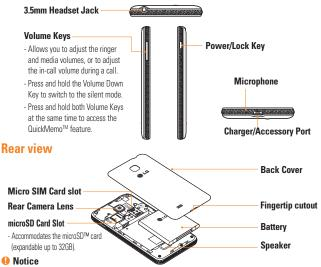
The NFC antenna for this model is on the back cover. This back cover is the only one that is offered with the model.
