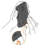
2 Gently insert the microSD card into the slot. Make sure the gold contact area is facing downwards.
