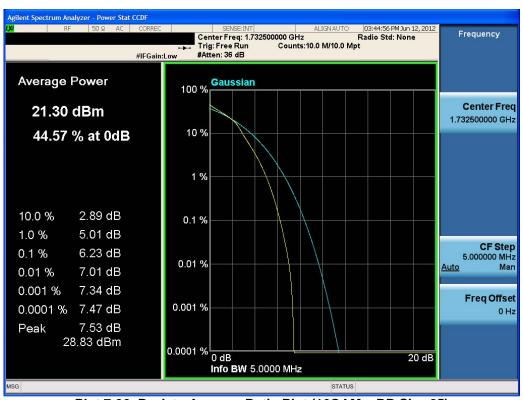
Plot 7-30. Peak to Average Ratio Plot (16QAM - RB Size 25)
