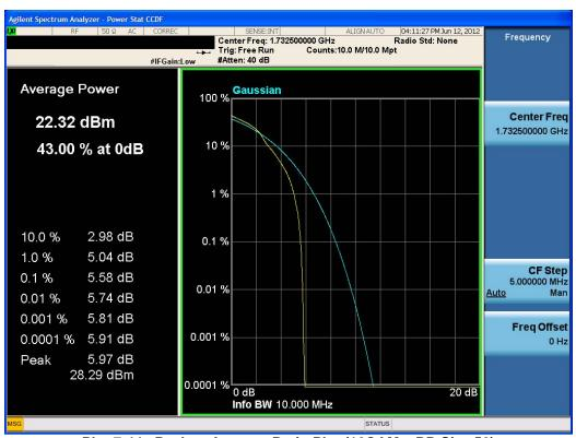
Plot 7-44. Peak to Average Ratio Plot (16QAM - RB Size 50)
