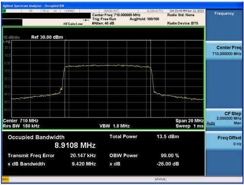
Plot 7-15. Occupied Bandwidth Plot (QPSK - RB Size 50)
