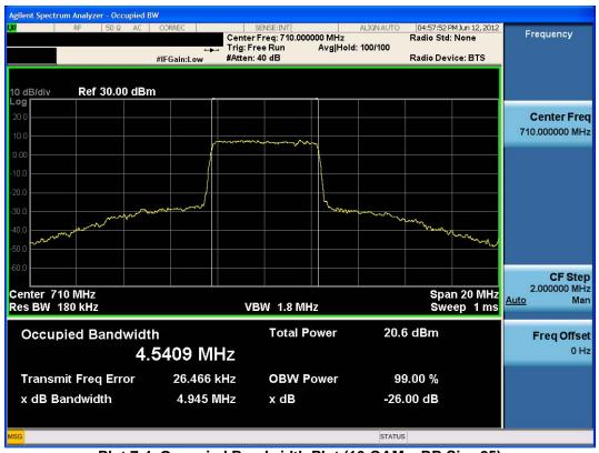
Plot 7-4. Occupied Bandwidth Plot (16-QAM - RB Size 25)
