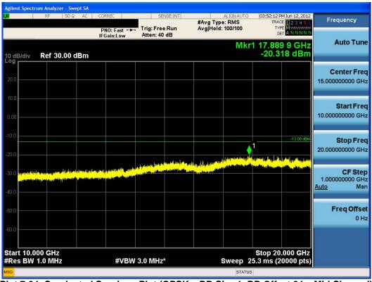
Plot 7-34. Conducted Spurious Plot (QPSK - RB Size 1, RB Offset 24 - Mid Channel)
