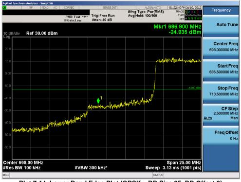
Plot 7-14. Lower Band Edge Plot (QPSK - RB Size 25, RB Offset 0)
