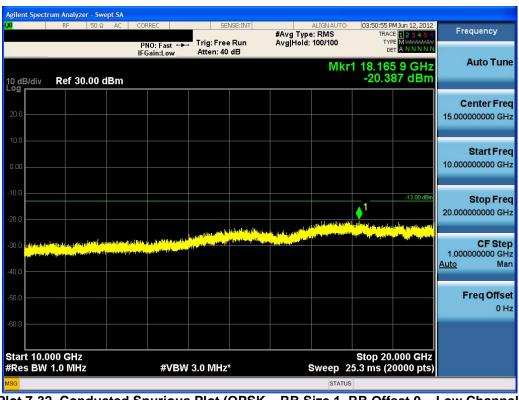
Plot 7-32. Conducted Spurious Plot (QPSK - RB Size 1, RB Offset 0 - Low Channel)
