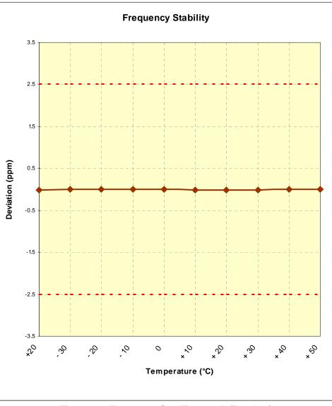
Figure 6-1. Frequency Stability Graph (Band 17)
