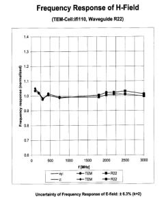
Figure 5-4 H-Field Probe Frequency Response
