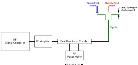
Figure 7-8 System Check Setup
