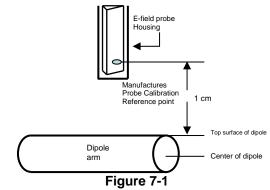
Separation Distance from Dipole to Field Probe
