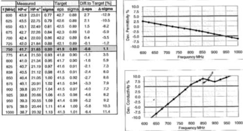
Figure 4-4 750MHz Head Tissue Equivalent Matter
