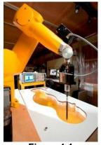
Figure 4-1 SAR Measurement System
