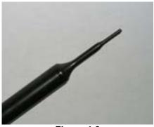
Figure 4-2 Near-Field Probe
