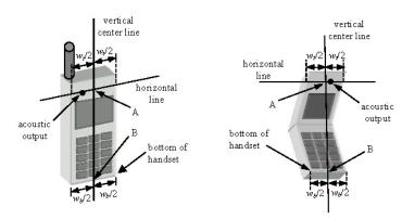
Figure 6-3 Handset Vertical Center & Horizontal Line Reference Points
