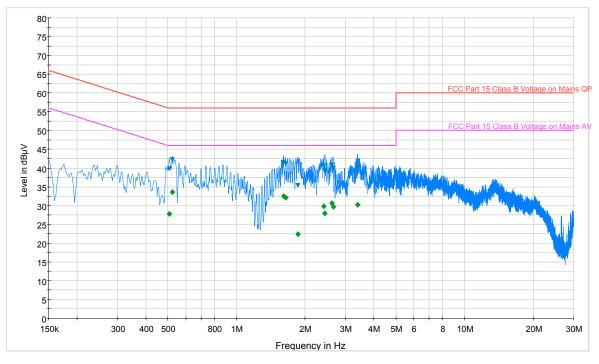
FCC Part 15 Class B Voltage on Mains QP.LimitLine Final Result 1-QPK FCC Part 15 Class B Voltage on Mains AV.LimitLine Preview Result 1-PK+ Final Result 2-AVG
