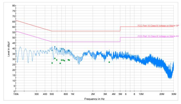
FCC Part 15 Class B Voltage on Mains QP.LimitLine Final Result 1-QPK FCC Part 15 Class B Voltage on Mains AV.LimitLine Preview Result 1-PK+ Final Result 2-AVG •
