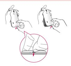
2 Slide the SIM card into the SIM card slot. Make sure the gold contact area on the card is facing downwards.
