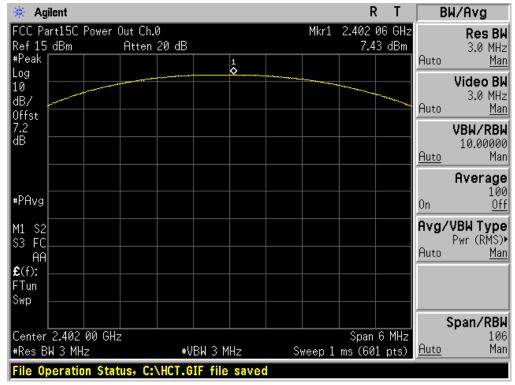
Test Plots (π/4DQPSK) Peak Power (Mid-CH)
