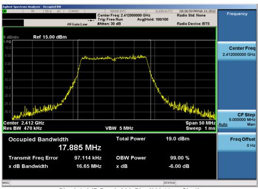
Plot 6-4. 6dB Bandwidth Plot (802.11g - Ch. 1)
