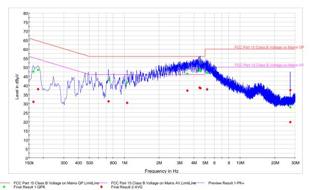
Plot 6-31. Line Conducted Plot with 802.11b (L1)
