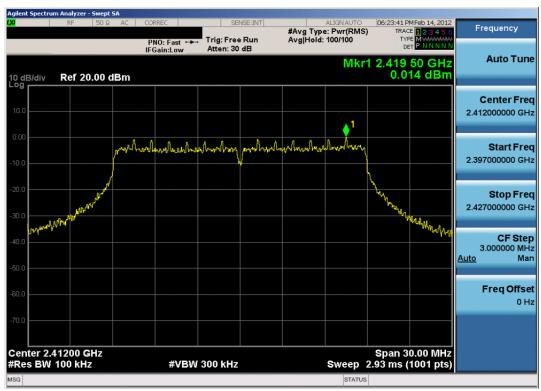
Plot 6-16. Power Spectral Density Plot (802.11n – Ch. 1)
