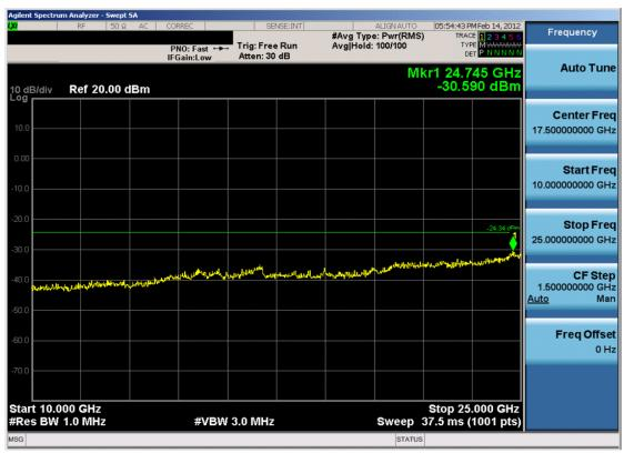
Plot 6-26. Conducted Spurious Plot (802.11b - Ch. 1)
