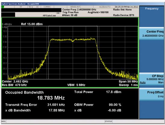
Plot 6-9. 6dB Bandwidth Plot (802.11n - Ch. 11)
