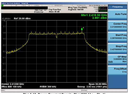
Plot 6-13. Power Spectral Density Plot (802.11g - Ch. 1)
