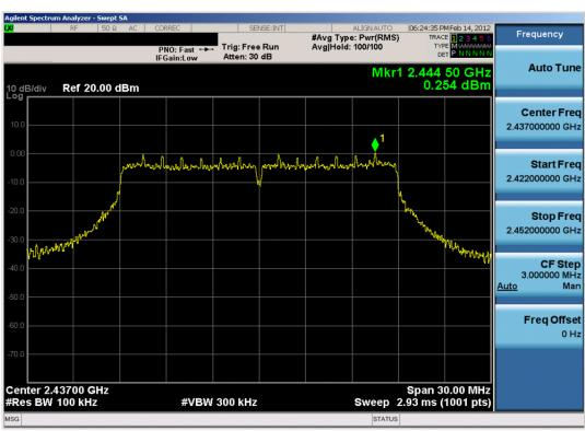
Plot 6-17. Power Spectral Density Plot (802.11n - Ch. 6)
