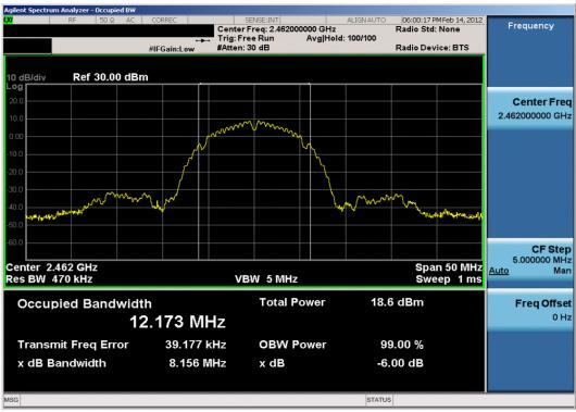
Plot 6-3. 6dB Bandwidth Plot (802.11b - Ch. 11)
