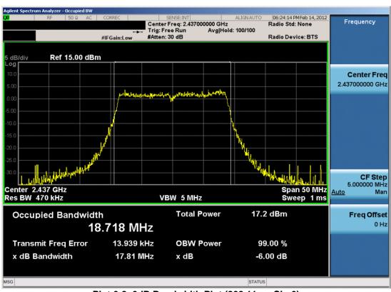
Plot 6-8. 6dB Bandwidth Plot (802.11n - Ch. 6)
