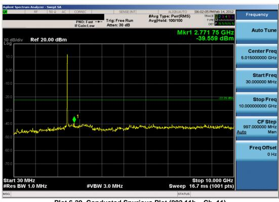
Plot 6-29. Conducted Spurious Plot (802.11b - Ch. 11)
