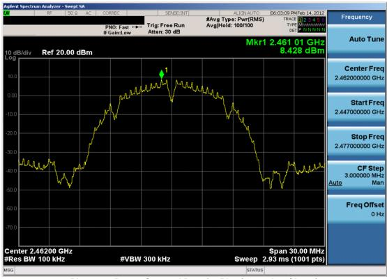
Plot 6-12. Power Spectral Density Plot (802.11b - Ch. 11)
