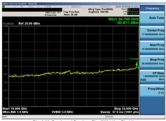
Plot 6-30. Conducted Spurious Plot (802.11b - Ch. 11)
