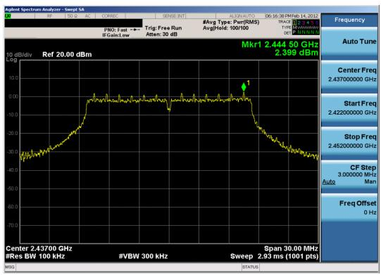
Plot 6-14. Power Spectral Density Plot (802.11g - Ch. 6)
