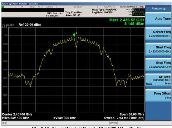
Plot 6-11. Power Spectral Density Plot (802.11b - Ch. 6)
