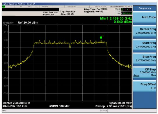
Plot 6-18. Power Spectral Density Plot (802.11n - Ch. 11)
