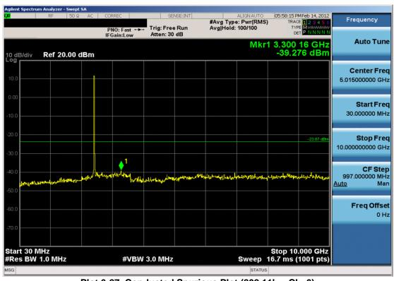
Plot 6-27. Conducted Spurious Plot (802.11b - Ch. 6)
