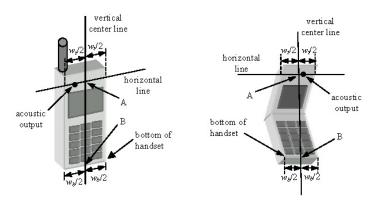
Figure 5-3 Handset Vertical Center & Horizontal Line Reference Points
