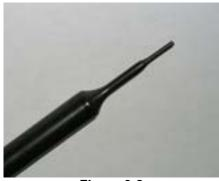
Figure 3-2 Near-Field Probe
