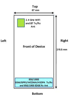
Figure 1-1 **DUT Antenna Locations**
