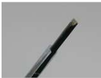
Figure 3.2 EX3DV4 E-field Probe
