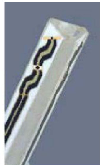
Figure 3.3 Probe Thick-Film Technique
