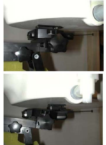
Figure 6.8 Body Belt Clip & Holster Configurations
