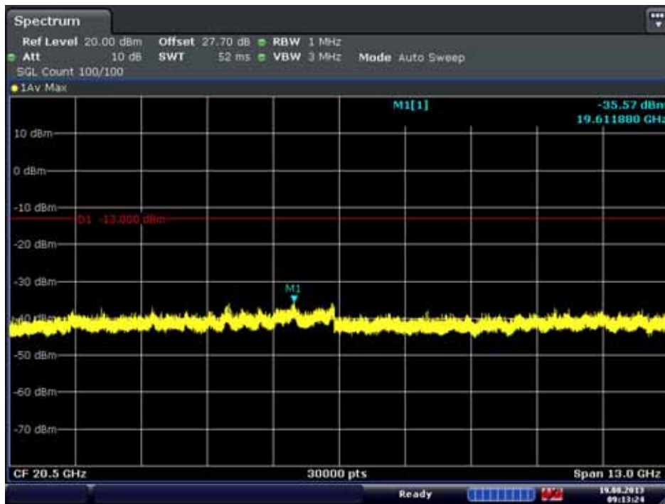
Conducted Spurious Plot 2 (10MHz QPSK - RB Size 1, RB Offset 0 - Mid Channel)
