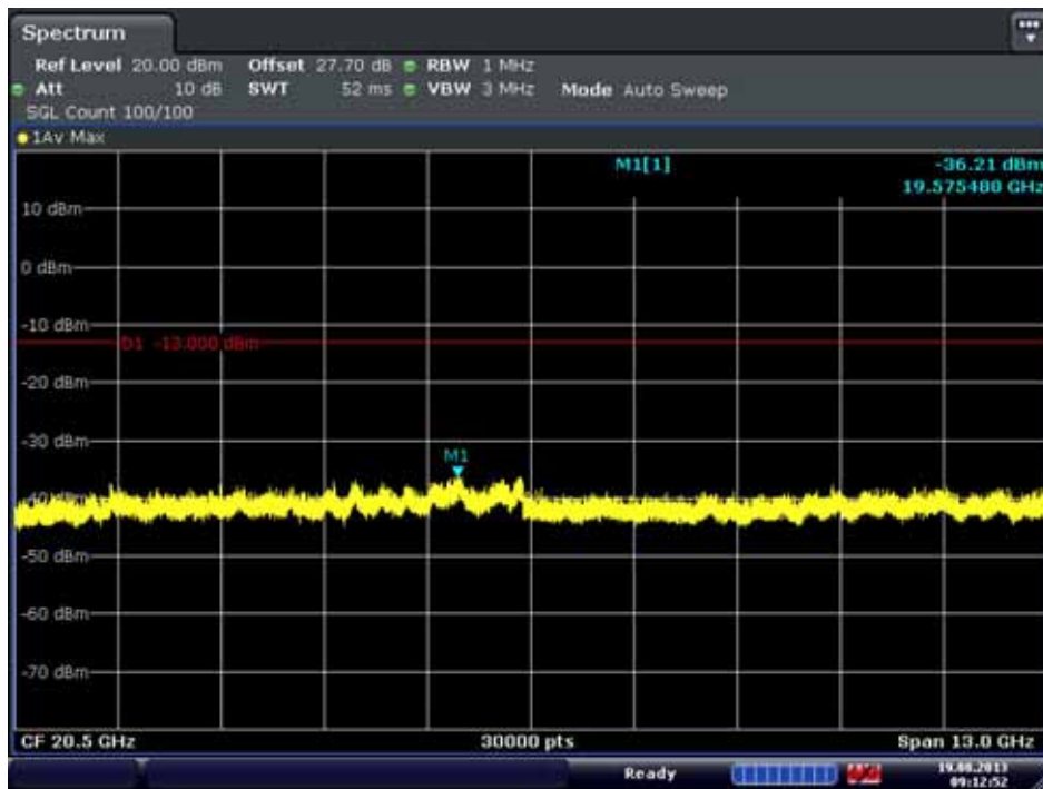
Conducted Spurious Plot 2 (10MHz QPSK - RB Size 1, RB Offset 0 - Low Channel)
