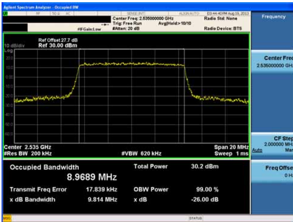
Occupied Bandwidth Plot (10MHz 16-QAM - RB Size 50)
