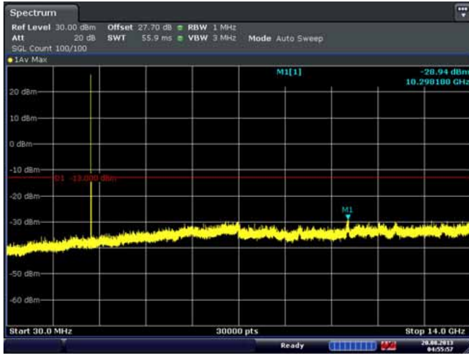
Conducted Spurious Plot 1 (5MHz QPSK - RB Size 1, RB Offset 0 - High Channel)
