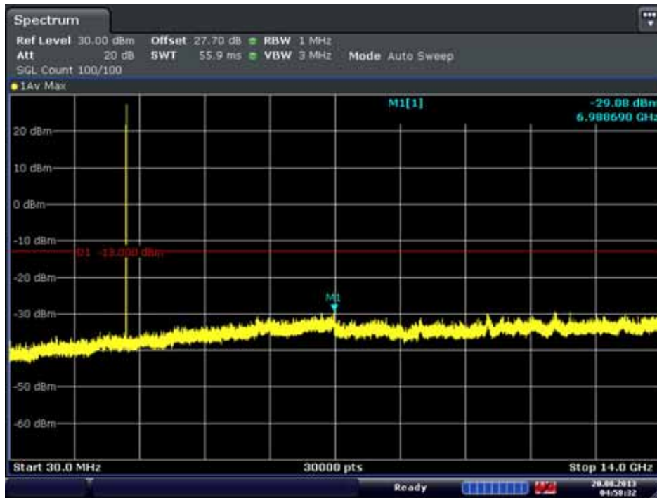
Conducted Spurious Plot 1 (5MHz QPSK - RB Size 1, RB Offset 0 - Mid Channel)
