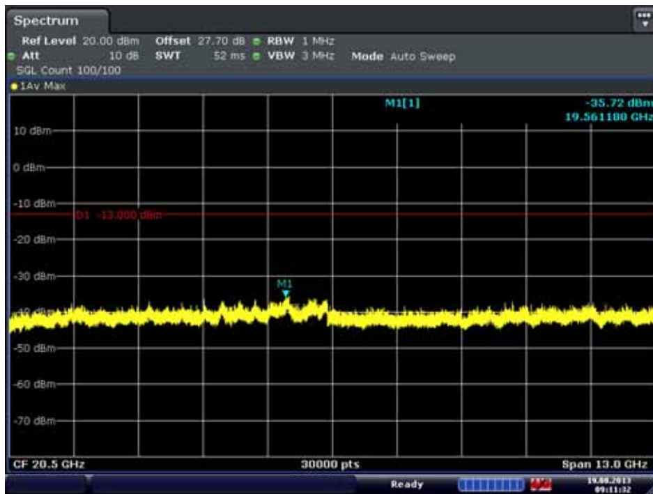
Conducted Spurious Plot 2 (5MHz QPSK - RB Size 1, RB Offset 0 - High Channel)
