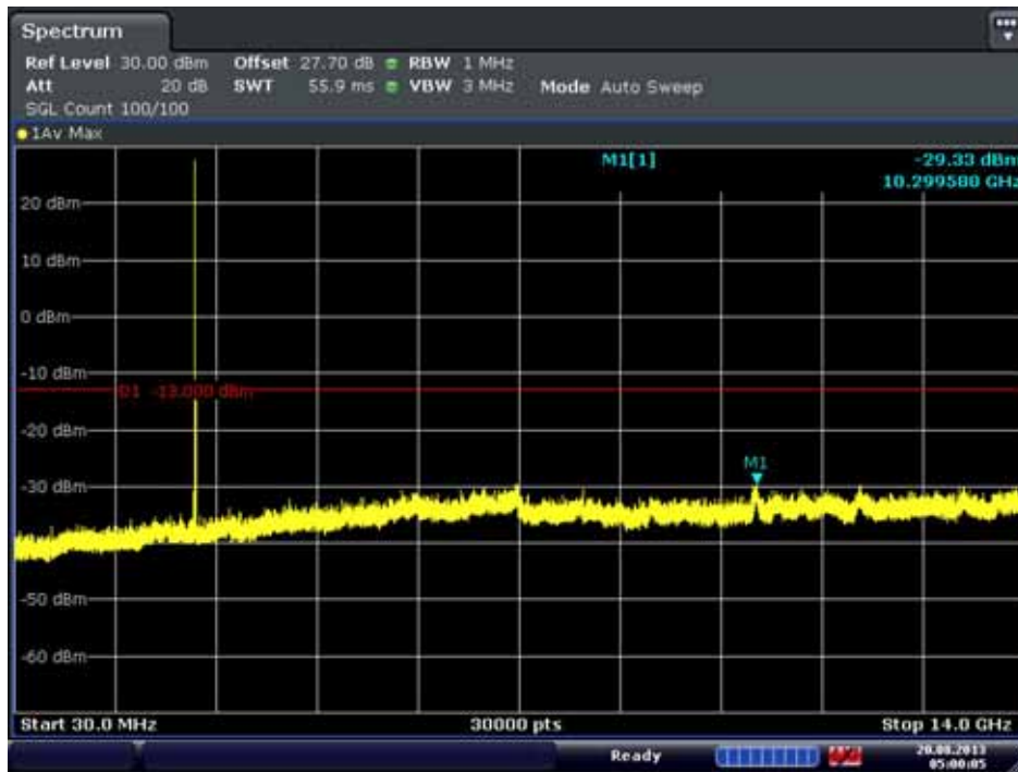
Conducted Spurious Plot 1 (10MHz QPSK - RB Size 1, RB Offset 0 - Mid Channel)
