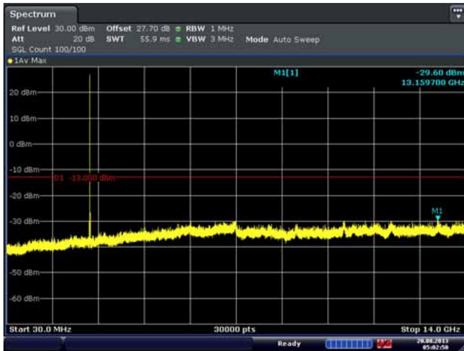
Conducted Spurious Plot 1 (10MHz QPSK - RB Size 1, RB Offset 0 - High Channel)
