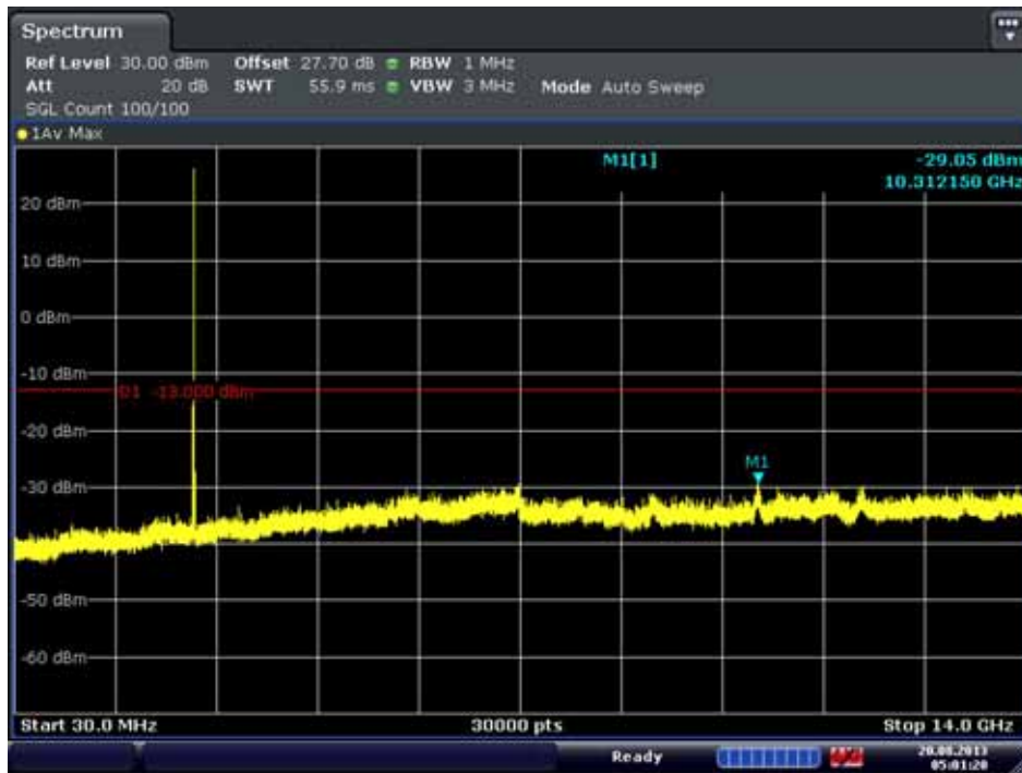
Conducted Spurious Plot 1 (10MHz QPSK - RB Size 1, RB Offset 0 - Low Channel)
