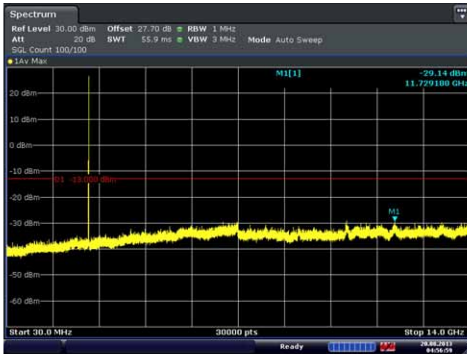
Conducted Spurious Plot 1 (5MHz QPSK - RB Size 1, RB Offset 0 - Low Channel)
