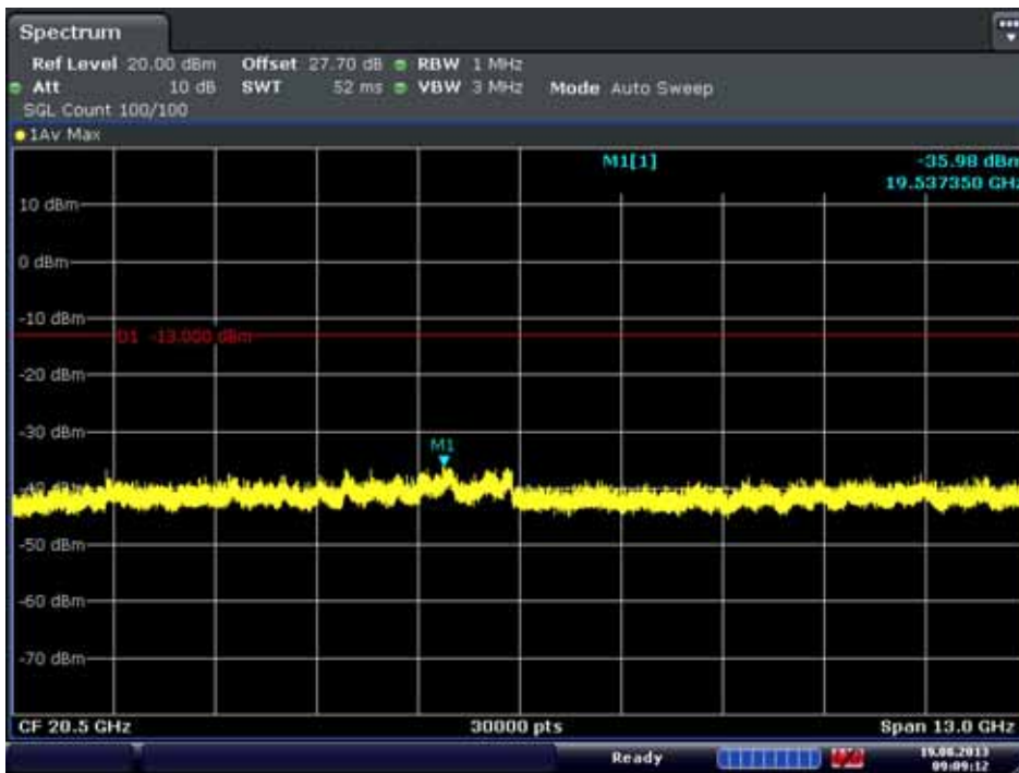
Conducted Spurious Plot 2 (5MHz QPSK - RB Size 1, RB Offset 0 - Low Channel)
