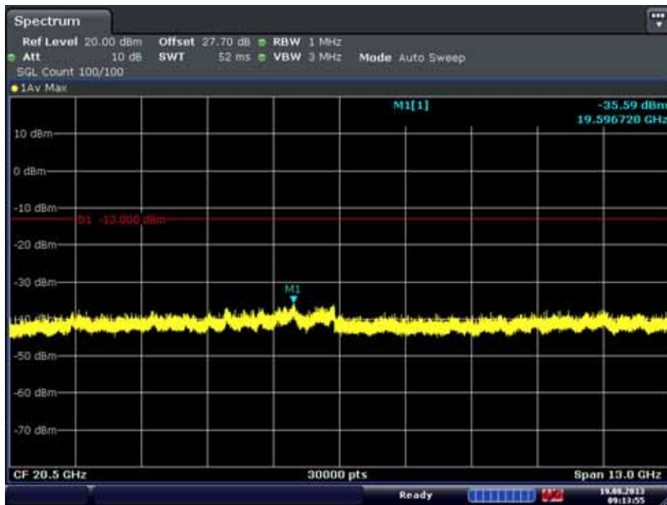
Conducted Spurious Plot 2 (10MHz QPSK - RB Size 1, RB Offset 0 - High Channel)
