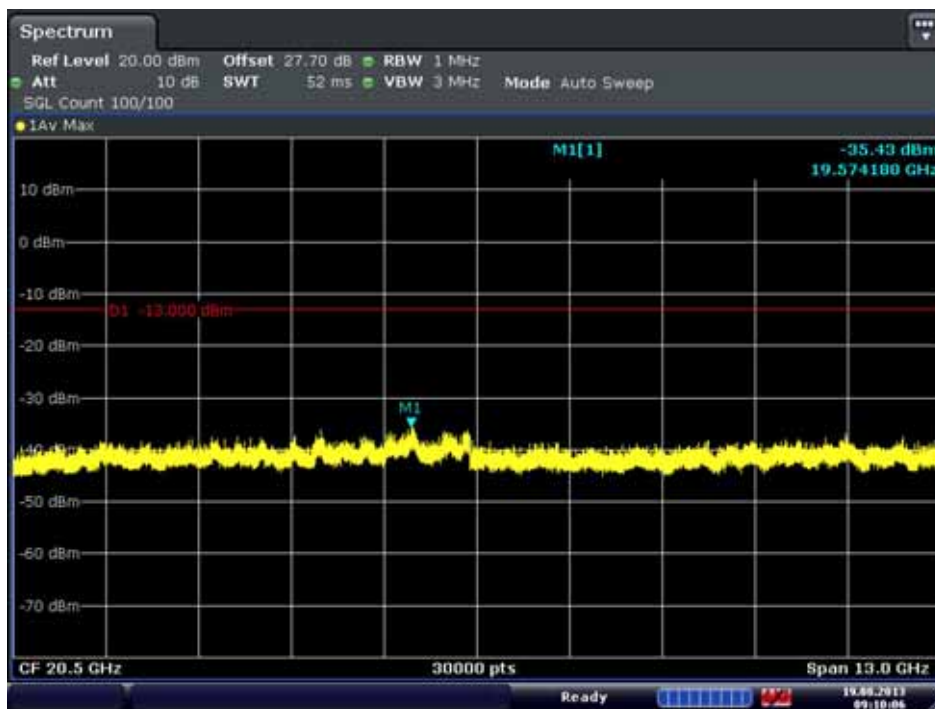
Conducted Spurious Plot 2 (5MHz QPSK - RB Size 1, RB Offset 0 - Mid Channel)
