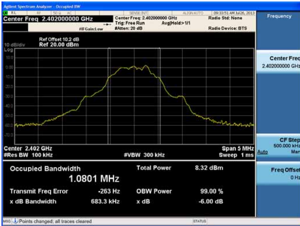
6dB Bandwidth plot (Low-CH 0)
