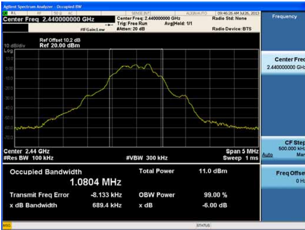
6dB Bandwidth plot (Mid-CH 19)
