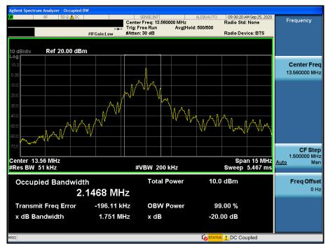
Note1: The 20 dB bandwidth was measured at all data rate and the worst case data was reported (This test item was tested at 424 kbps.)
