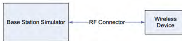
Figure 9.1 Power Measurement Setup
