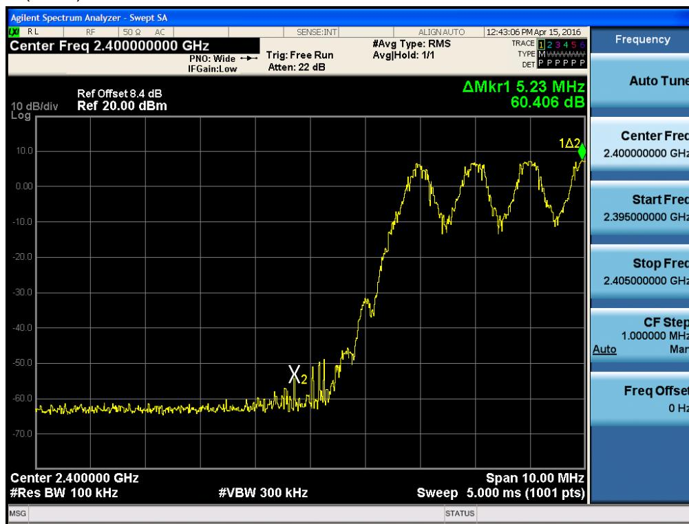
Test Plots with hopping (GFSK)
