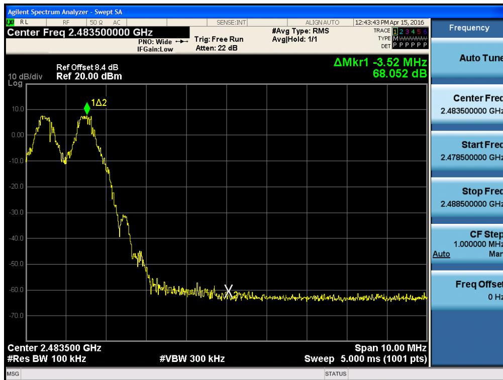
Test Plots with hopping (8DPSK)
