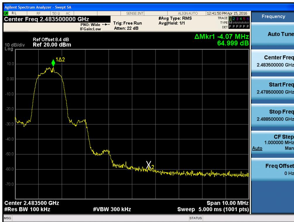
Test Plots with hopping (GFSK)
