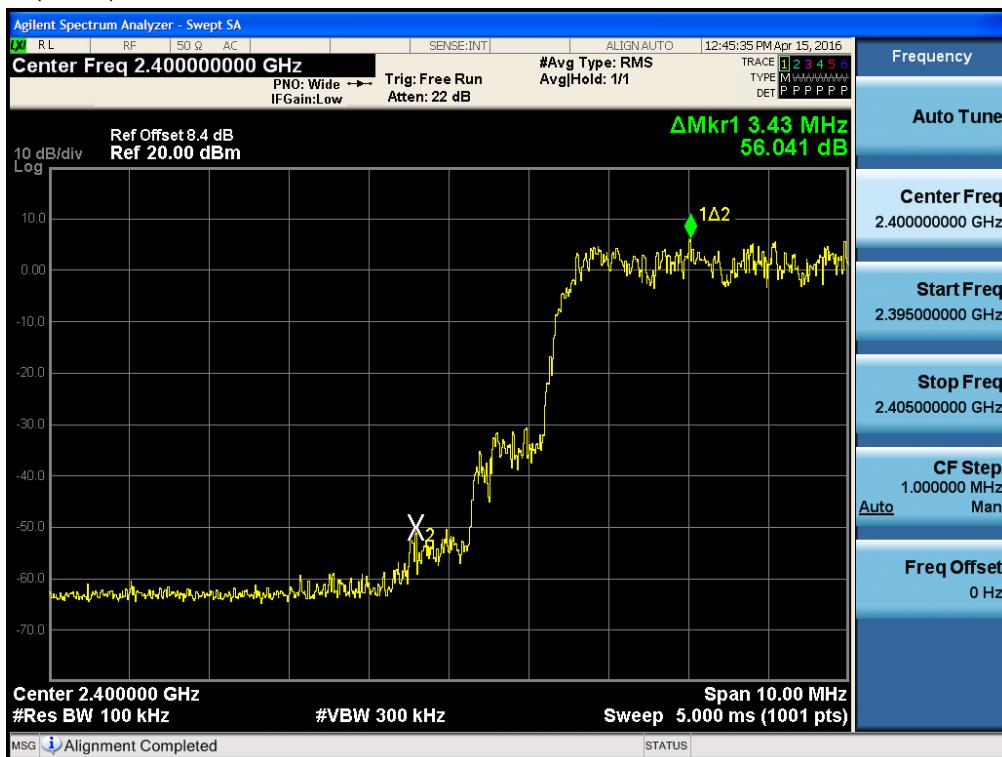
Test Plots with hopping (8DPSK)
