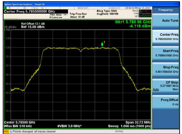
802.11ac_VHT20UNII 3 BAND PSD CH 157
