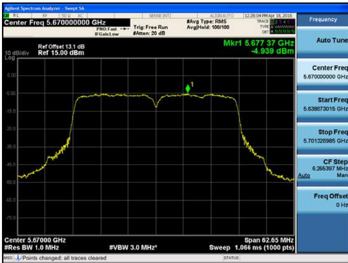
802.11ac_VH40UNII 2C BAND PSD CH 134
