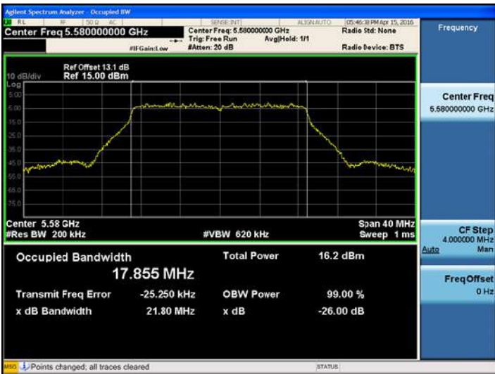
802.11ac_VHT20UNII 2C BAND 26dB Bandwidth(CH 116)
