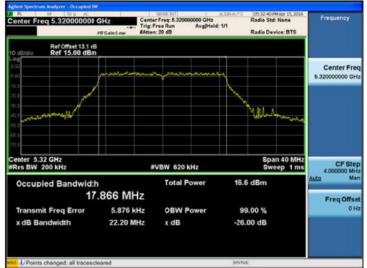
802.11n_HT20UNII 3 BAND 26dB Bandwidth(CH 149)
