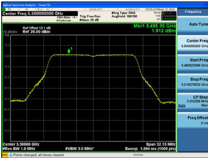
802.11a UNII 2C BAND PSD CH 100
