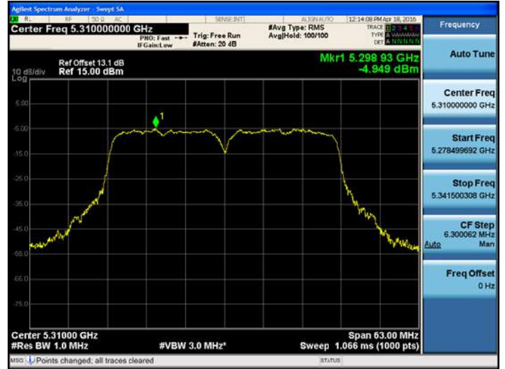
802.11ac_VHT40UNII 3 BAND PSD CH 151
