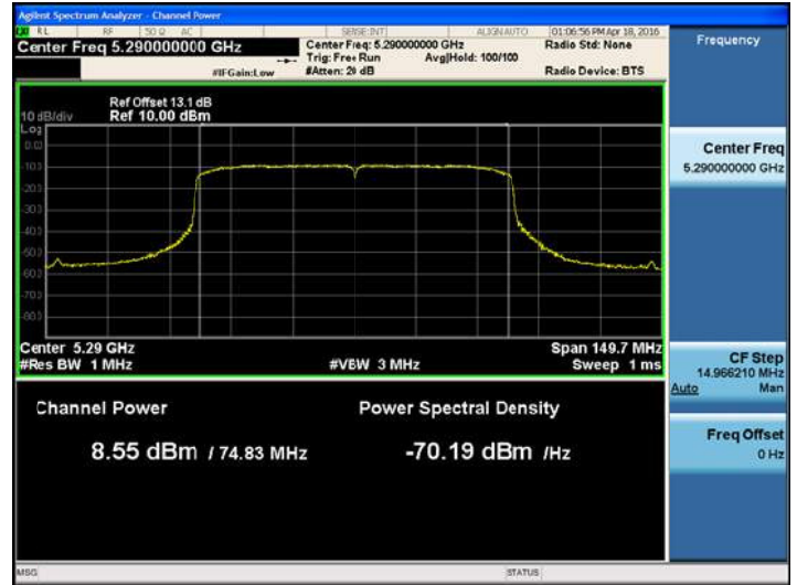
802.11ac_VHT80 UNII 3 BAND Average Power (5755 MHz) CH 155 MCS3
