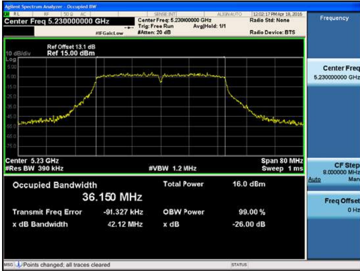
802.11ac_VHT40UNII 2C BAND 26dB Bandwidth(CH 110)
