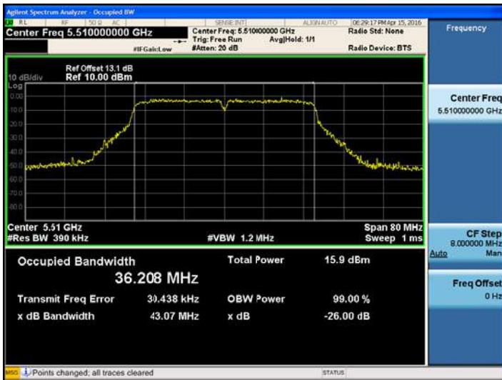
802.11n_HT40UNII 2C BAND 26dB Bandwidth(CH 102)
