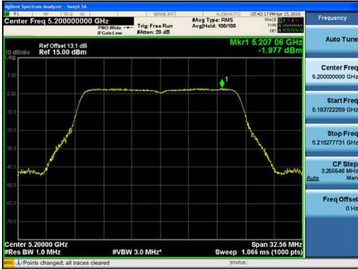
802.11ac_VHT20UNII 2C BAND PSD CH 116
