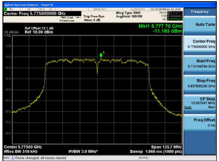
802.11ac_VHT80UNII 3 BAND PSD CH 155
