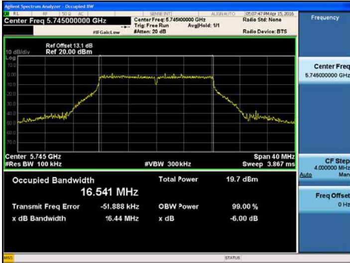
802.11ac_VHT20 UNII 3 BAND 6dB Bandwidth(CH.157)
