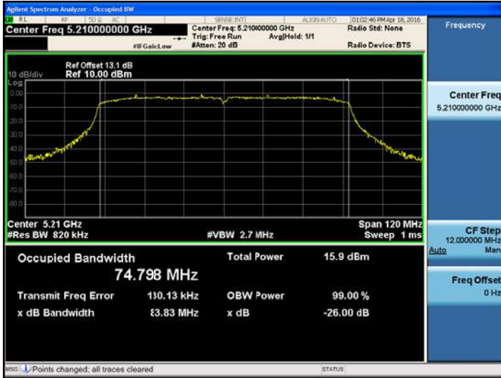
802.11ac_VHT80UNII 2C BAND 26dB Bandwidth(CH 106)
