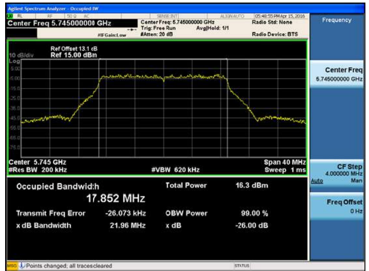
802.11ac_VHT20UNII 3 BAND 26dB Bandwidth(CH 149)
