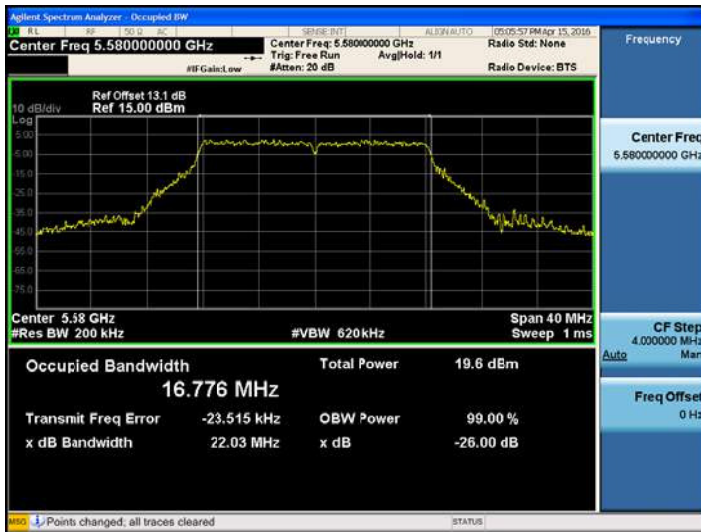
802.11a UNII 2C BAND 26dB Bandwidth (CH116)
