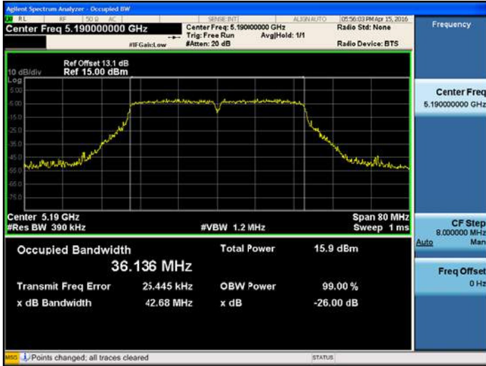
802.11n_HT40UNII 2C BAND 26dB Bandwidth(CH 102)
