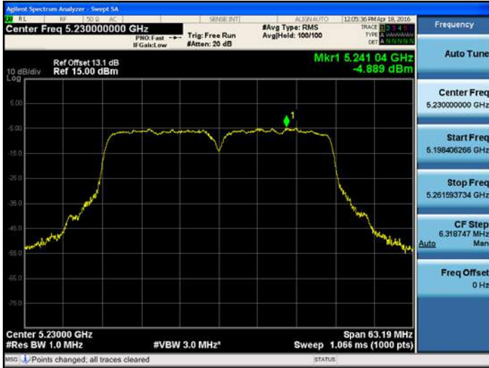
802.11ac_VH40UNII 2C BAND PSD CH 134
