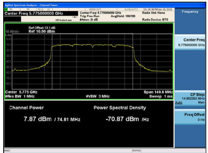
802.11ac_VHT80 UNII 3 BAND Average Power (5755 MHz) CH 155 MCS3
