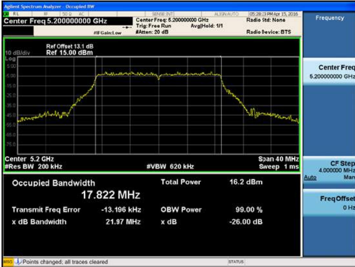
802.11n_HT20UNII 2C BAND 26dB Bandwidth(CH 100)
