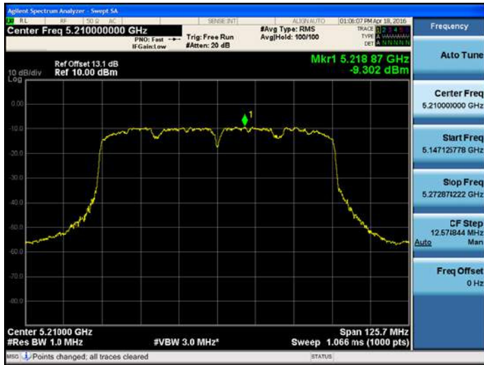
802.11ac_VHT80UNII 2C BAND PSD CH 106
