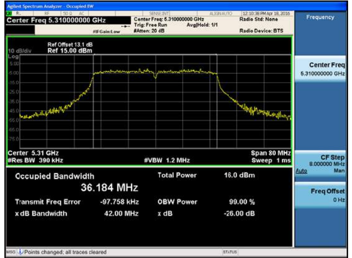
802.11ac_VHT40UNII 3 BAND 26dB Bandwidth (CH 159)
