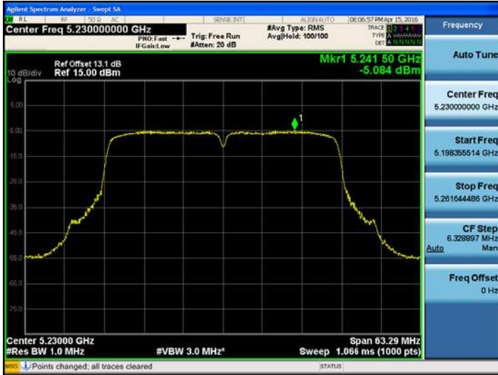
802.11n_HT40 UNII 2C BAND PSD CH 134
