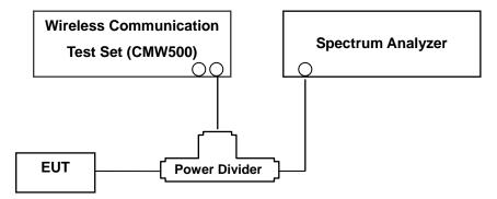
(Configuration of conducted Emission measurement) Test Procedure
