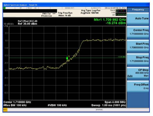
Band Edge Plot (10 MHz BW, QPSK, AWS Band 4 - Low Channel)
