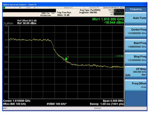
Band Edge Plot (10 MHz BW, QPSK, PCS Band 2 – High Channel)
