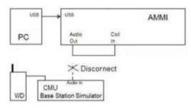
Figure 10: Signal Verification Setup
