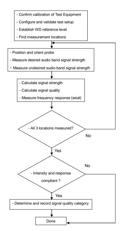
Figure 6: T-Coil measurement flowchart
