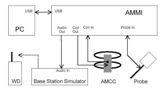
Figure 2: T-Coil setup cabling.
