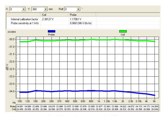
Figure 3: Frequency Response measured in AMCC
