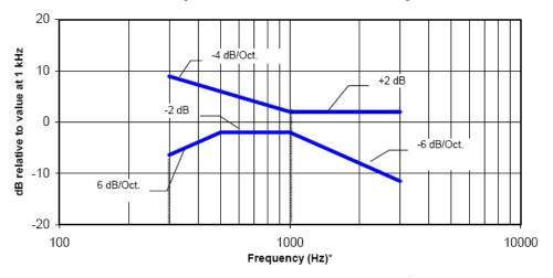
Figure 4 : Magnetic field frequency response for WDs with a field ≤ −15 dB (A/m) at 1 kHz
