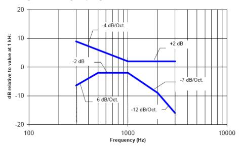
Figure 5: Magnetic field frequency response for WDs with a field that exceeds -15 dB(A/m) at 1 kHz
